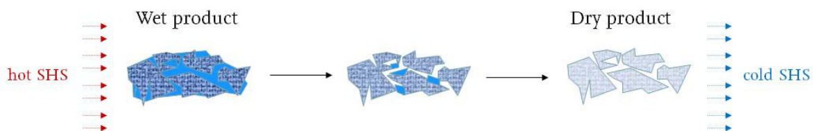
Figure 1.1: Simplified process visualization of convective drying with superheated steam
