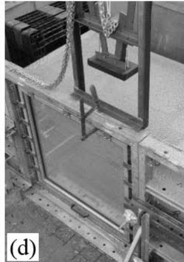
Guided freefall weights with variable basic shapes and falling heights up to 1.2m
