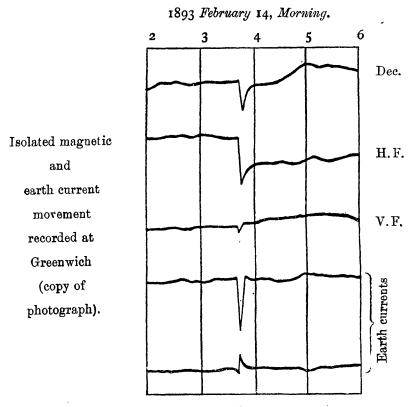
accompanied by corresponding marked earth-current, the different elements all being in a quiescent state both before and after the little outbreak. It may be further noted that the diagram indicates increase of declination and of horizontal and vertical force, the movements being in this respect in harmony with the usual Greenwich direction of first movement in storms, as shown in Table II.
