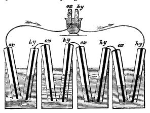
axis of the tube platinized platina foil, which in the battery I constructed was about one-fourth of an inch wide. It is obvious that, by allowing the platina to touch the liquid, the latter would spread over its surface by capillary action and expose an extended superficies to the gaseous atmosphere. The battery was charged with dilute sulphuric acid, sp. gr. 1.2, and the following effects were produced :---
