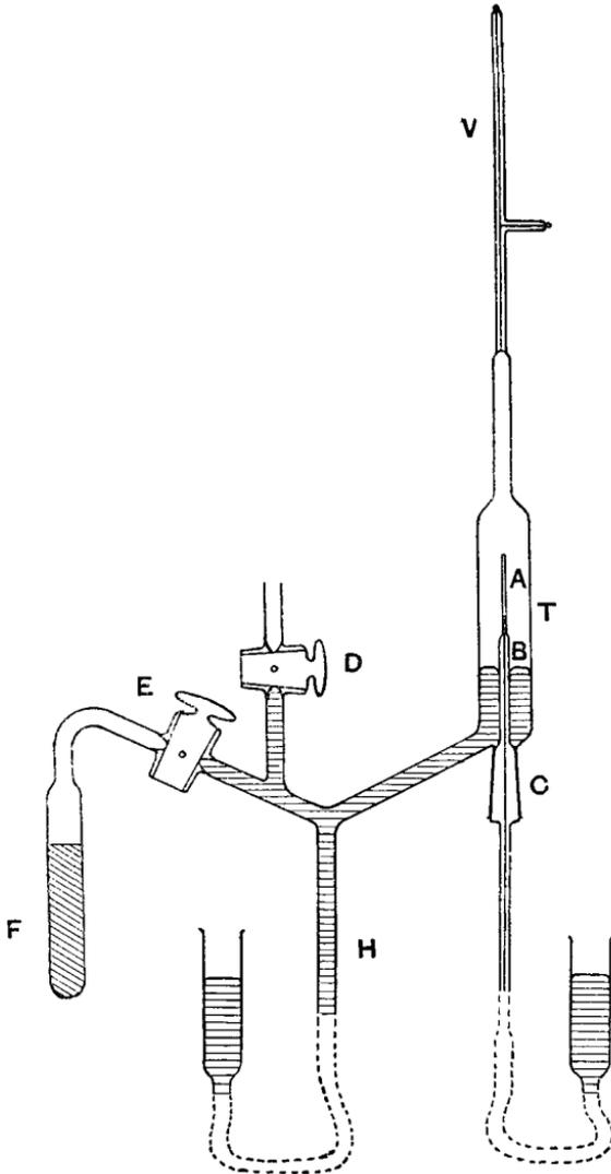
mercury-column into a fine glass tube A about 1.5 cms. long. This fine tube, which was sealed on a larger capillary tube B, was sufficiently thin to allow the  $\alpha$  particles from the emanation and its products to escape, but sufficiently strong to
