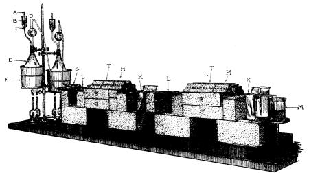
Fig. 1.--Apparatus for the determination of arsenic.
