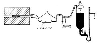
The decomposition tube consisted of a piece of Jena glass tubing of about 16 mm. bore, and 14 in. long, sealed at one end, and heated in a horizontal electric tube furnace wound with nichrome ribbon. The furnace was calibrated by means of a platinum-platinum rhodium thermocouple, and the heating current plotted against the temperature. A constant heating zone of 3 in. was obtained in the middle of the furnace.
