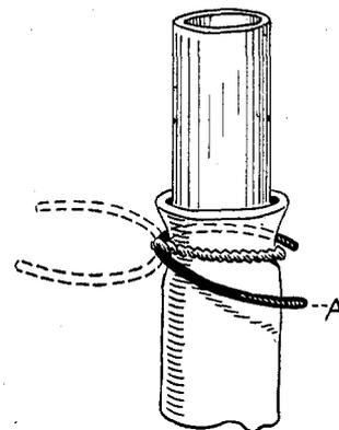
A further advantage of this mode of attachment lies in the ease with which it may be dismantled, requiring as it does no pliers or other tools for this purpose.
