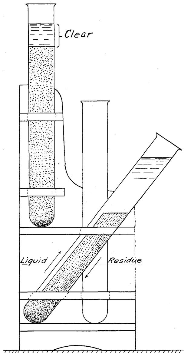
The decanting operation can thus be finished in one-third of the time required by the usual method of using vertical tubes. It is common practice to use narrow inclined tubes, etc., for obtaining a rapid decanting in liquids or for separating dust from air. The same principle can, as shown, be of use in the laboratory.
