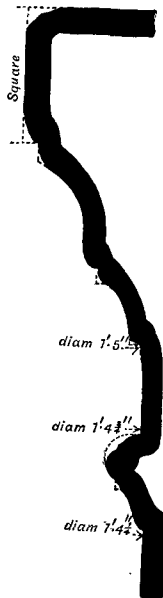
Fig. 4. Section of capital of column from peristyle of House No. 3. ( \frac{1}{8} linear.)
