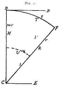
a tangent to the circle, and u is the angular velocity of revolution, *i.e.*, the linear velocity of a point on r at the distance of unity from C.
