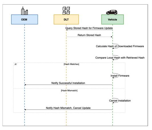
After downloading, the vehicle calculates the hash of the downloaded firmware and compares it with the hash value stored on the DLT network. If the hash values match, the vehicle proceeds with the installation process, as shown in Figure 5.
