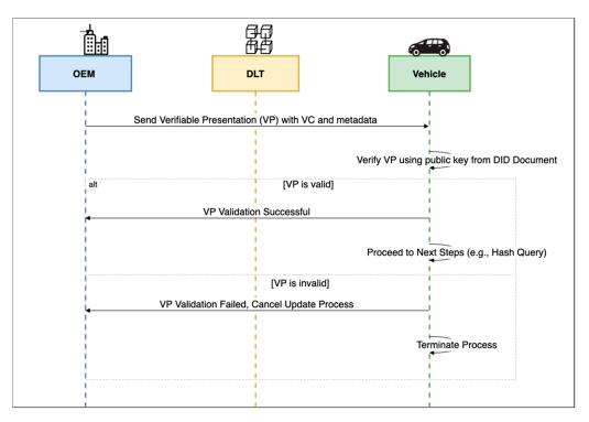
Figure 4. Sequence diagram for verifying VP.
