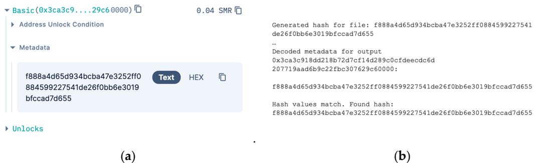
Figure 6. Process of downloading and verifying firmware hash values: (a) shows the metadata field in the IOTA explorer where the hash is displayed; (b) illustrates the vehicle comparing its local firmware hash with the hash retrieved from the DLT.
