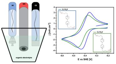
Figure 1 Schematic representation of the three-electrode setup and comparison of CVs 3,3 S<sub>2</sub>V and 3,4 S<sub>2</sub>V at scan rate 500 mV.s<sup>-1</sup>.
