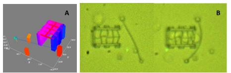
**Figure 2** Proof of concept of containers with a flexible barrier (manual control). (A) CAD model. (B) Process of micromanipulation with optical tweezer: gate open (left); gate closed; three live cells placed to the container (right).
