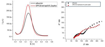
Figure 1 Differential pulse voltammetry (DPV) gaph compared to Nyquist diagram after measurement with interferent (albumin).
