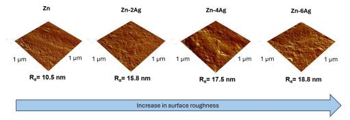
Figure 1 AFM image of Zn and Zn-Ag surface (1x1 µm).
