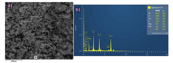
Figure 1 SEM photography - a), and EDXRF spectrum of the sludge sample after precipitation - b).
