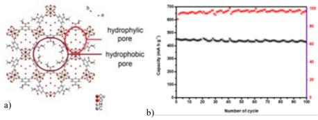
Figure 1 a) A view of hydrophobic and hydrophilic pores present in the STAM-1 framework and b) changes of capacity for S/STAM-1/Super P/PVDF electrode at 0.5 C (100 cycles).
