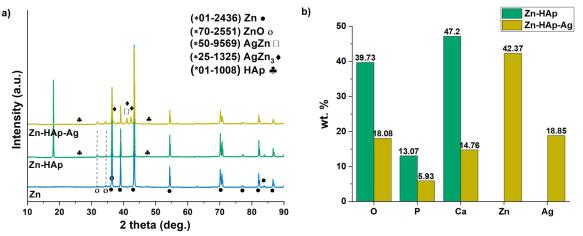
Figure 1 XRD spectrum (a) and elements content from EDS area analysis of Zn-HAp and Zn-HAp-Ag (b).
