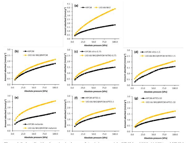
**Figure 1** Carbon dioxide adsorption isotherms of a) pristine materials (HPCM and UiO-66-NH<sub>2</sub>) and HPCM un/dopped/composite materials of b) unmodified HPCM, nitro sample containing c) 0.75 mmol and d) 1.5 mmol of functional groups, e) melamine, APTES with content of f) 1 mmol and g) 10 mmol.
