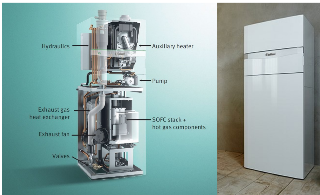
Figure 2: Structure of the current XellPower FC heating unit: the fuel cell system with the auxiliary units is in the bottom, the auxiliary condensing gas boiler heater is on top. © Vaillant (left picture). Vaillant micro CHP (right picture) [17].
