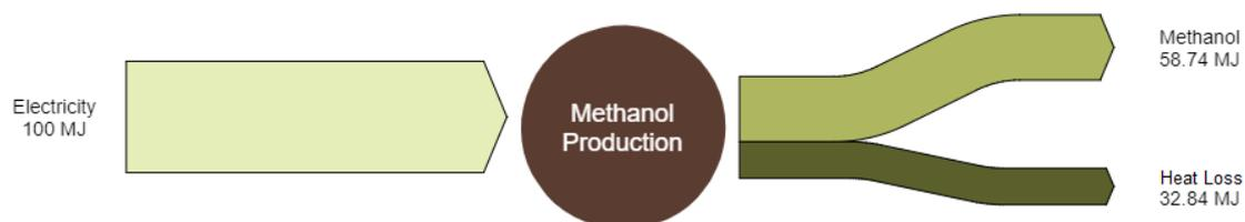
Figure 2 Methanol from Power Energy Balance
