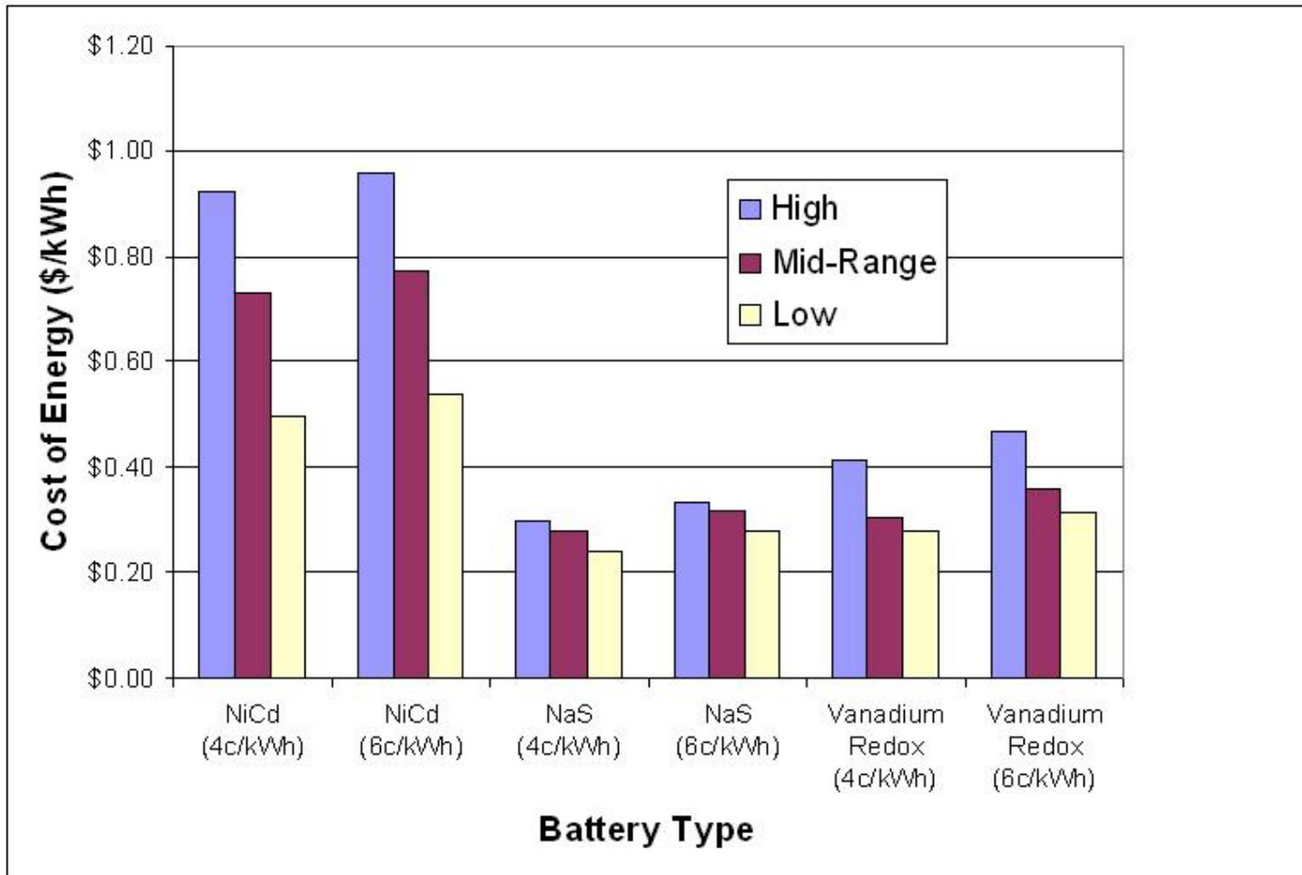
The cost of NiCd batteries is high in comparison to sodium sulfur and Vanadium Redox batteries due to relatively high capacity (\$/kWh) costs.
