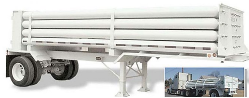
Figure 21: Trailer and storage is same vessel.
