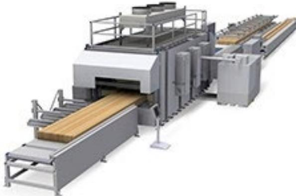
Figure 2: Kallesøe timber press [2]
