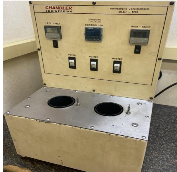
[Fig.3: Atmospheric Consistometer Used to Condition Slurry]
