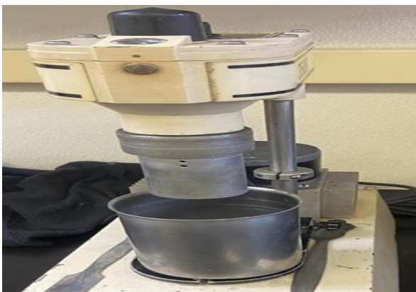
[Fig.2: Viscometer Used for Rheology]
