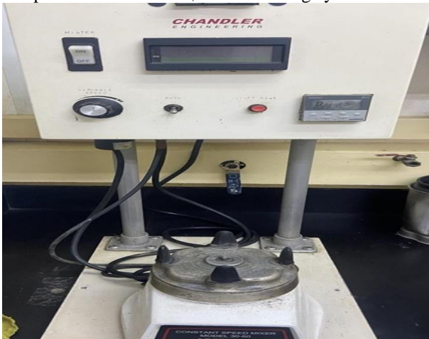
[Fig.1: Mixer Blender Used to Mix Cement Slurry]
