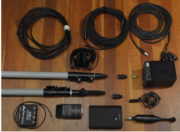
Figure 2. PIRMS Components (clockwise from top left) power cable, headphones, XLR, soundfield mic cable, loudspeaker, mic shockmount, soundfield microphone, battery, Zoom H6 Recorder, direct box, two painter’s poles, and various adapters.
