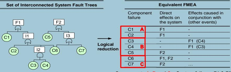
Components A, B and C – System failures F1 & F2
