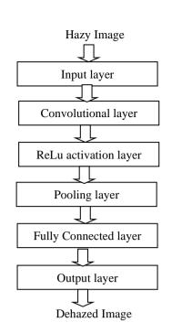
[Fig.2: Block Diagram of Convolutional Neural Network]
