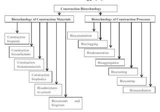
[Fig.1: Directions of Construction Biotechnology, Source:] [2]
