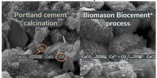
[Image 1: Comparison Between Chemical Process of Portland Cement and Biocement, Source:] [14]
