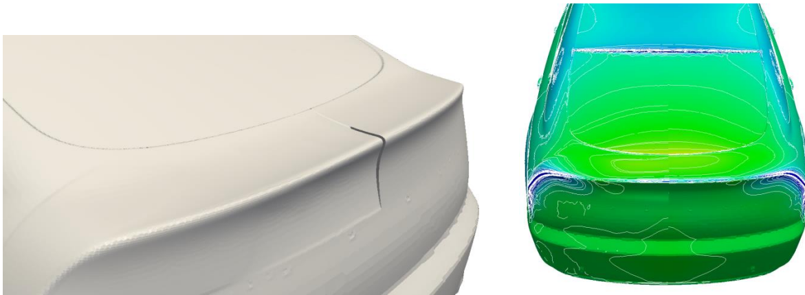
Fig. 6: Comparison between the optimised (left half of the car) and starting (right half) rear part geometries of the DrivAer model. On the right the pressure distribution for both the optimised and starting geometry is presented.
