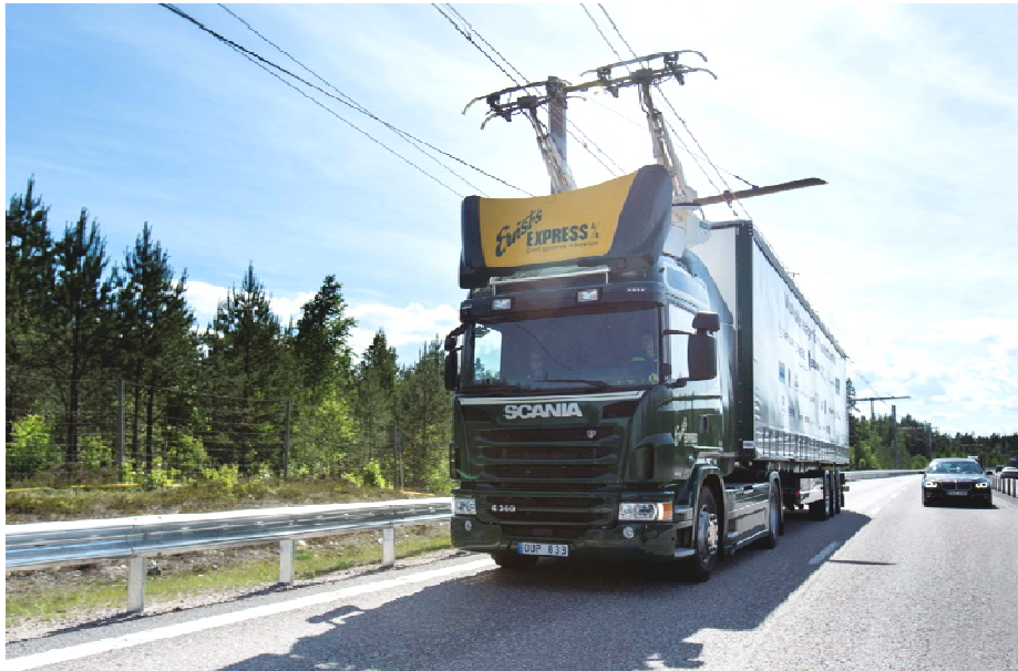
Fig. 2 Hybrid truck in electric operation on public road in Sweden
