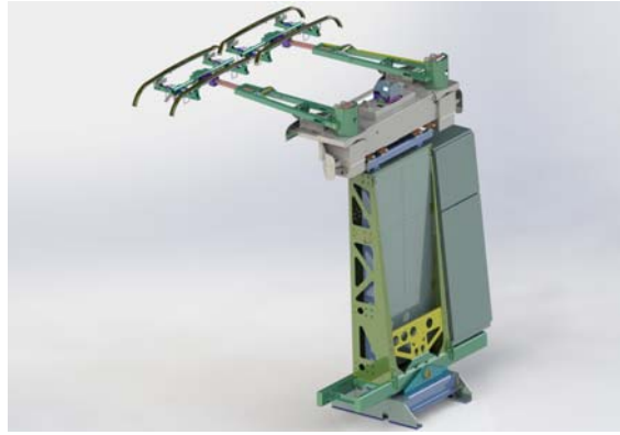
Fig. 4 Active Pantograph to connect with an Overhead-Contactline
