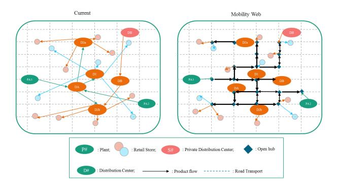
Fig 2 Example of current and potential future distribution network (adjusted, cf. ibid., p.28)
