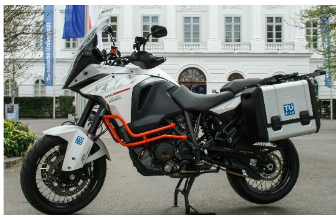
Figure 1 KTM 1290 Super Adventure equipped and instrumented as a Motorcycle Probe Vehicle (MoProVe)
