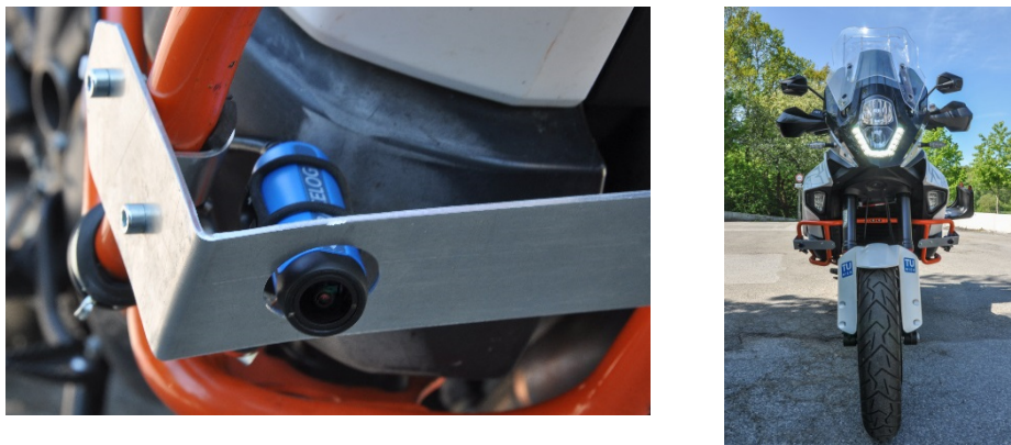
Figure 4 HD-camera system mounted on MoProVe.
