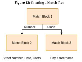
Matchers are trained upon initialization, before they are added to the entire tree. With the shown code, we first tell the CCC to create an initial matcher which is a Fingerprint matcher. We then add a Number matcher. This matcher is called when the main matcher predicts that the inserted data belongs to the 'number' class. If this is the case, than the data is send to this
