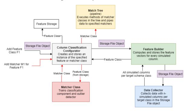
Figure 3: ARPSAS System Architecture
