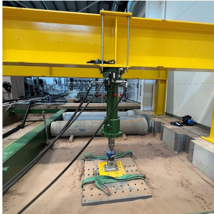
Figure 13. Automated loading system applying 110 kN cyclic load above a buried pipe joint
