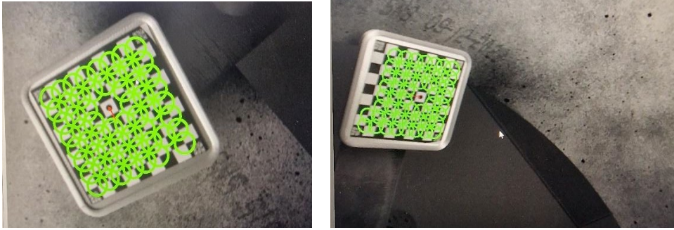
Figure 2. Calibration images for the DIC system, taken inside of a 300mm dia concrete pipe with bespoke calibration target
