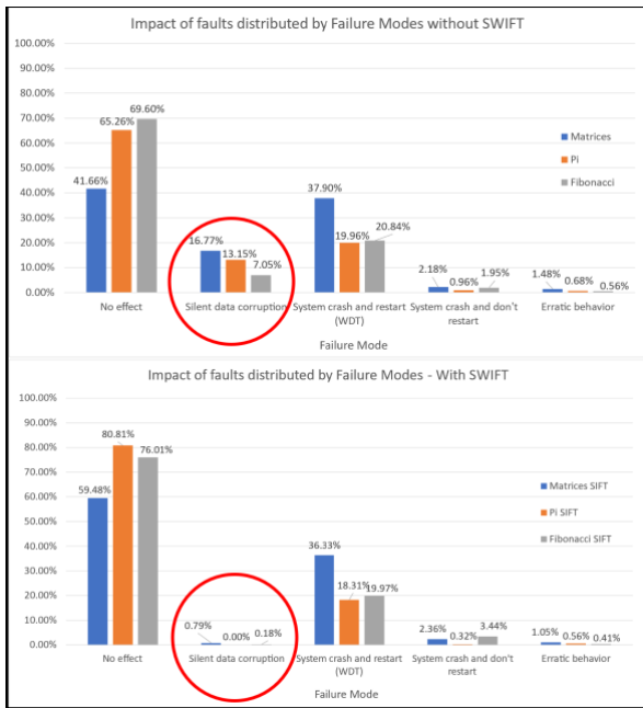
Fig. 8. Comparison of the impact of faults distributed by failure modes on the all the software tested before and after being strengthened with SWIFT techniques
