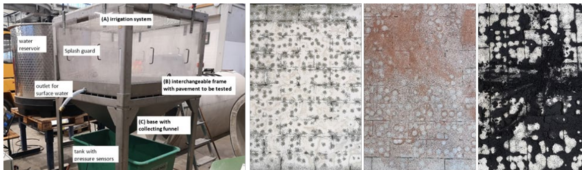
Figure 1.20. IKT irrigation system and different sediments tested over the permeable pavement surface.
