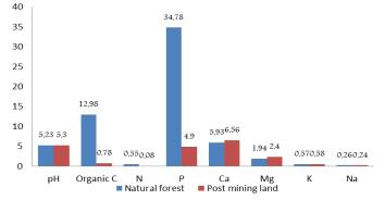
Figure 2. The change of soil chemistry properties on natural forest and post mining land; Description : pH (pH), organic C ( %), N (Nitrogen : %), P (Phosphorus : ppm), Ca (calcium : me/100 g), Mg (magnesium : me/100 g), K (pottasium: me/100 g), Na (sodium : me/100g).
