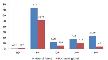
**Figure 1.** The change of soil physical propertieson natural forest and post mining land. Description : BD (Bulk density : gram/cm<sup>3</sup>), PR (Porosiys : %), DP (Drainage pore : %), AT (Available water: %) PM (Permeability : cm/hour).
