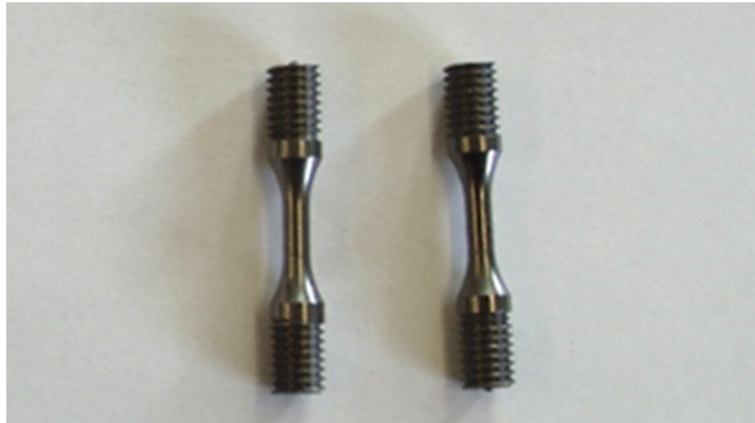
Figure 134. M6 specimens in MoGr for experimental characterization with the split-Hopkinson pressure bar.
