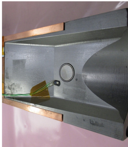
Figure 100. View of the downstream MoGr tapering of the CuCD jaw. No sign of damage to the component or to the BPM is evidenced.
