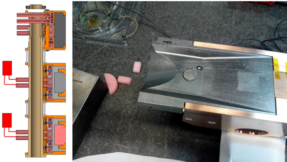
Figure 94. Left: water reservoir connections for the two HL-LHC jaws. Right: optical fibres on the CuCD jaw.
