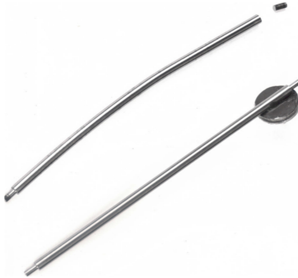
Figure 8. Beryllium rods damaged by an off-axis beam impact at the CERN SPS in the 1970s.
