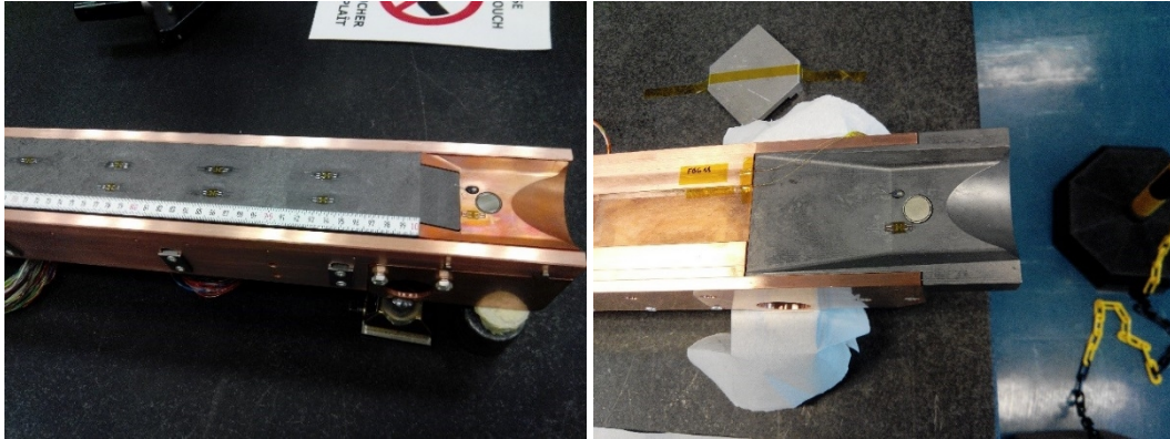
Figure 93. Strain gauges and temperature probes on CFC (left) and CuCD (right) jaws.
