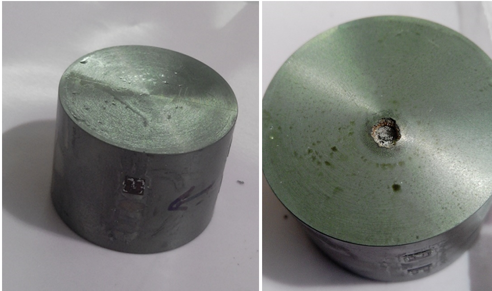
Figure 60. Upstream (left) and downstream (right) faces of the Inermet180 M6.2 specimen impacted by 2.7 \times 10^{12} protons at 440 GeV during the HRMT-14 experiment. The droplets on the upstream face come from the near specimen M6.1 , which was NEG-coated. Coating melted and deposited on M6.2 .
