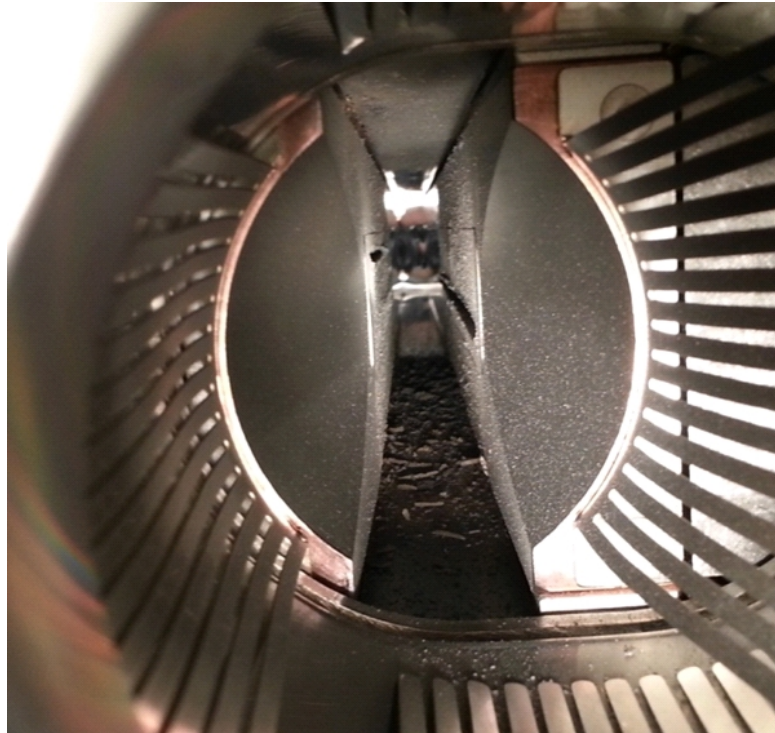
Figure 11. Effects of impact tests on LHC tungsten collimator, upstream view. Note the presence of two longitudinal grooves and extensive debris on the bottom of the vacuum chamber.
