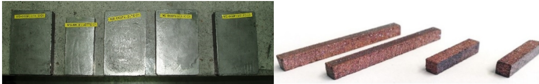
Figure 77. Left: MoGr plate for prototyping ( 150 \times 100 \times 25 \text{ mm}^3 ). Right: CuCD samples for bending tests.
