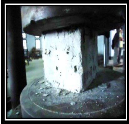
Plate-1:- Compressive strength test of plain concrete cubical specimen
