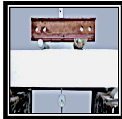
Plate-4:- Flexural strength test of SFRC beam specimen
