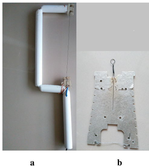
Figure 2. (a) Hot wire sponge cutter (For hand shape) (b) Hot wire sponge cutter for cylindrical channels
