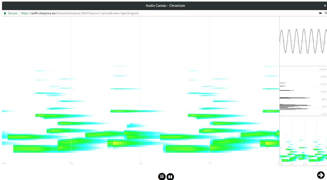
Figure 2: The DrAwME tool in visualization mode, with the selected view (here the spectrogram) in the middle and the visualization miniatures on the right side.
