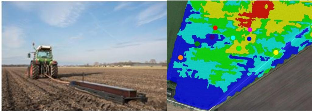
**Figure 5.** On the left, a tractor scanning the soil with the DualEM sensor. On the right, soil scan result of the pilot field in Netherlands in 2016.
