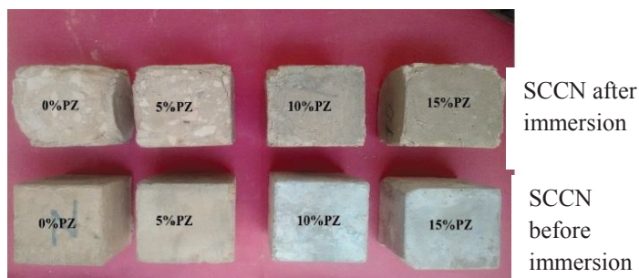
Figure 4: SCCN specimens degradation before and after immersion in 5%Na 2 SO 4 solution.
