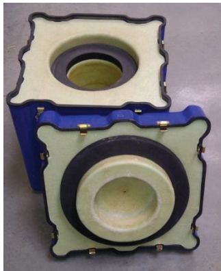
Figure 1: the QAB calibrated calorimeter used on concrete (left) and the non-calibrated calorimeter used on small sample (right).
