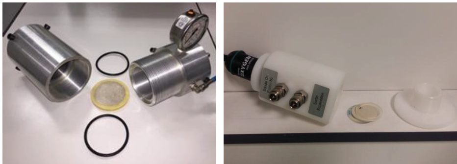
Figure 2: Overview of CO 2 (left) and O 2 (right) diffusion set-ups.
