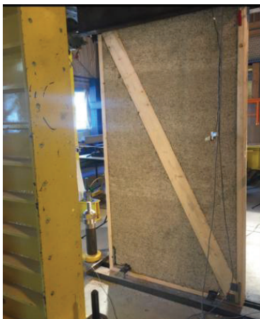
Figure 9: Diagonal bracing hemp walls in test.
