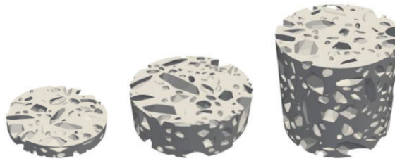
Figure 1: examples of specimens with thickness of 8 (left), 20 (middle) and 55 (right) mm.
