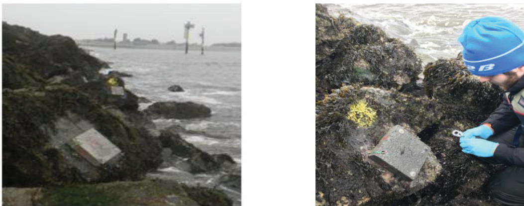
Figure 1: Concrete tiles installation and deployment.
