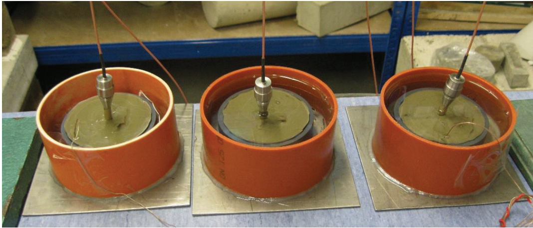
Fig. 2 Photo of placement of the AE sensors.
