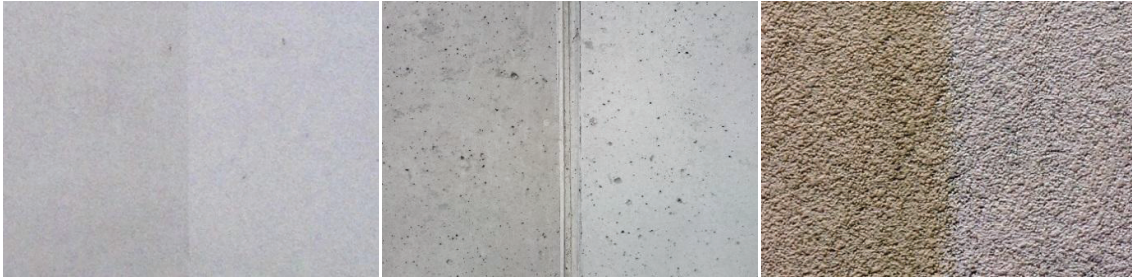
Figure 1: Light cleaning effect of BALCLEAN after 1 year of application on different cement containing surfaces.
