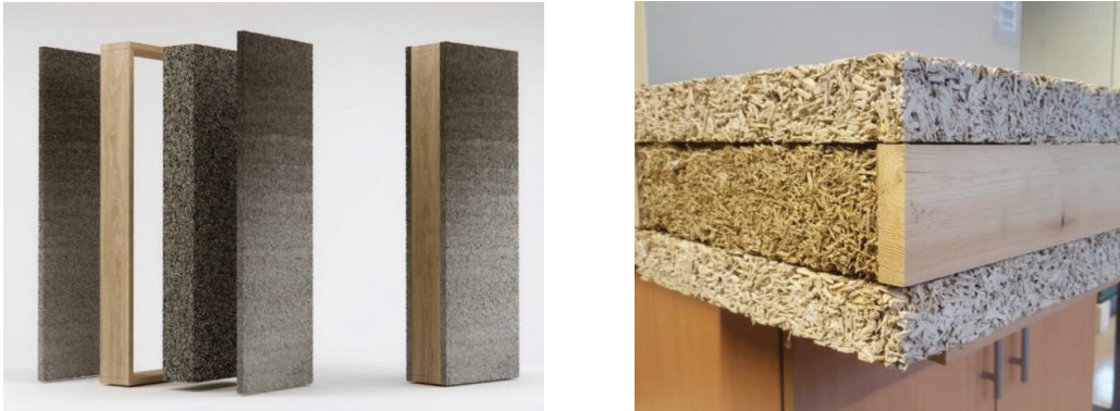
Figure 1: Proposed panel prototype with three different density layers (left), experimental panel scaled model (right)
