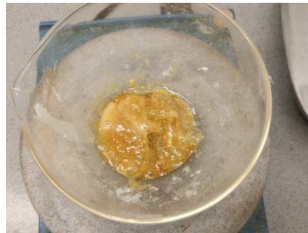
Figure 12: d) Melted polymer and PLA granulate.
