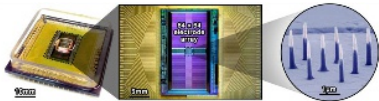
Fig. 27. CMOS nanoelectrode array for network intracellular recording. Adapted with permission from Refs. [88, 96], Springer Nature Ltd.
