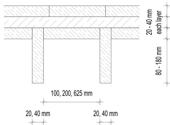
**Figure 5:** The XR-lam plate geometries selected for specimen production and testing
