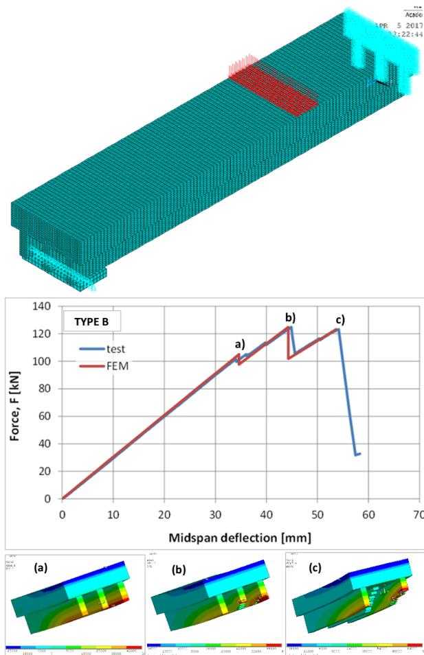
**Figure 11:** A combined 3D finite element model follows the gradual damage development
