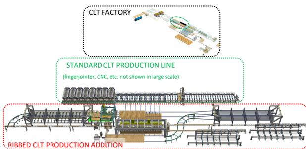
**Figure 13:** The XR-lam plate full industrial production line
