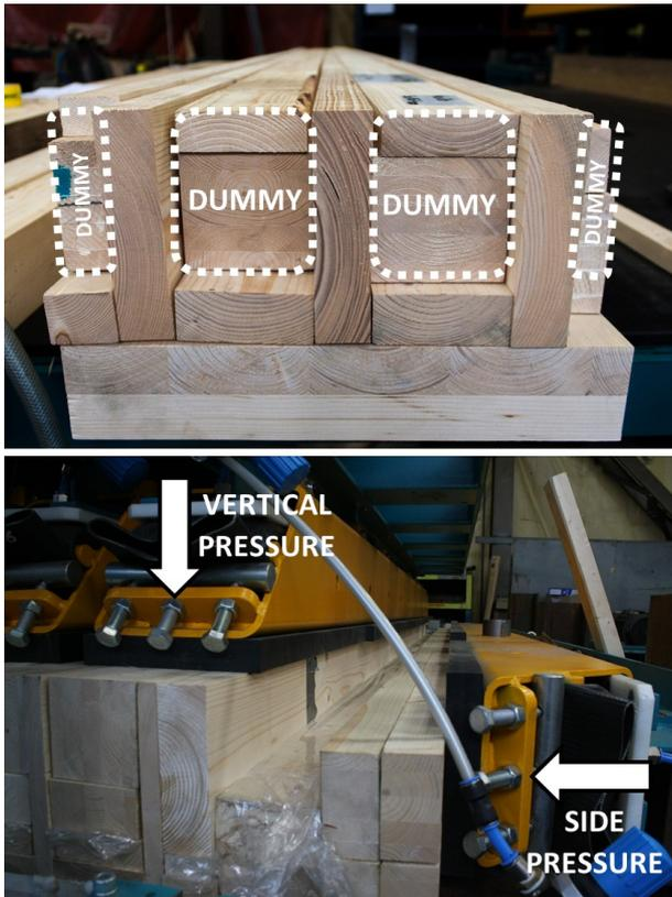
**Figure 6:** The temporary dummy elements used for pressing the ribbed structure and the pressing production
