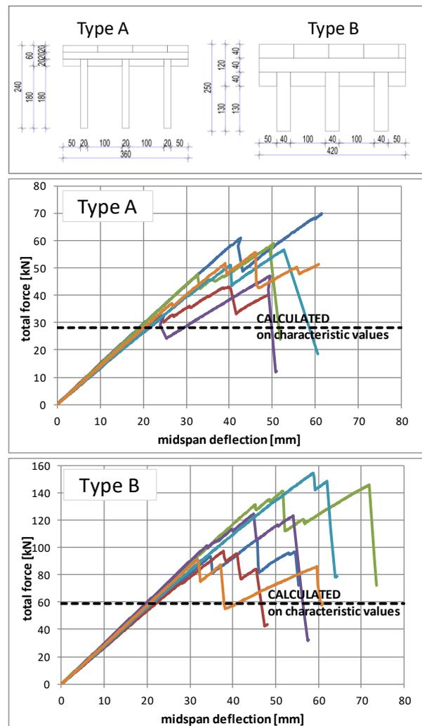
**Figure 8:** Load displacement curves and damage development for ribbed plates in out-of-plane bending
