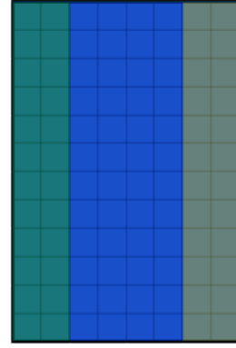
Fig. 4. A diagram of the cell layout of the 96-cell module modeled in this study. The three colors designate the cells belonging to each of the three bypass diodes.
