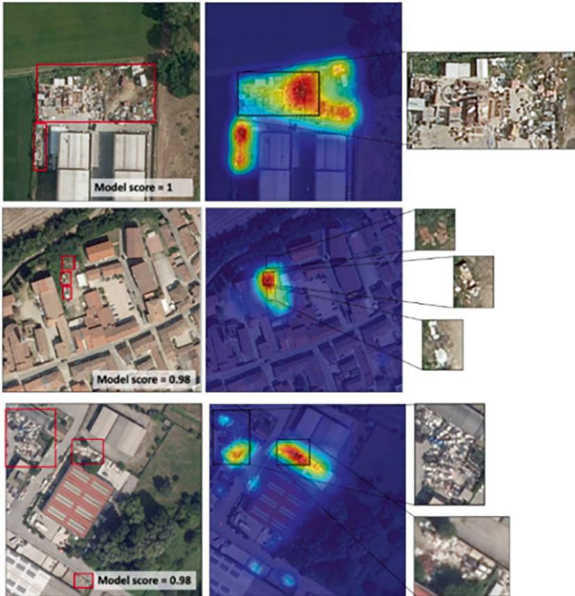
**Fig. 16.2** Examples of waste detection in remote sensing images by a Deep Learning model: images annotated by the detector with the confidence value (model score) about the presence of waste (left); images overlaid with Class Activation Maps that highlight the region where the detector has found waste (centre); zoom on the regions of interest containing waste dumps (right)
