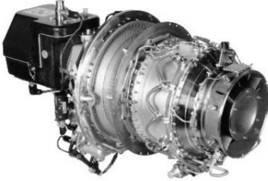
řekil 1: United Technologies Corporation, Pratt & Whitney Aircraft PW206 turbo prop motoru
