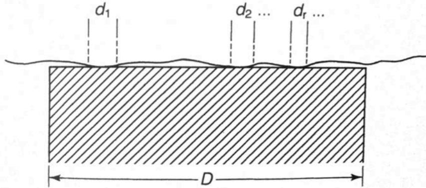
Figure 13 Imperfect contact between ice and structure (Sanderson 1988)
