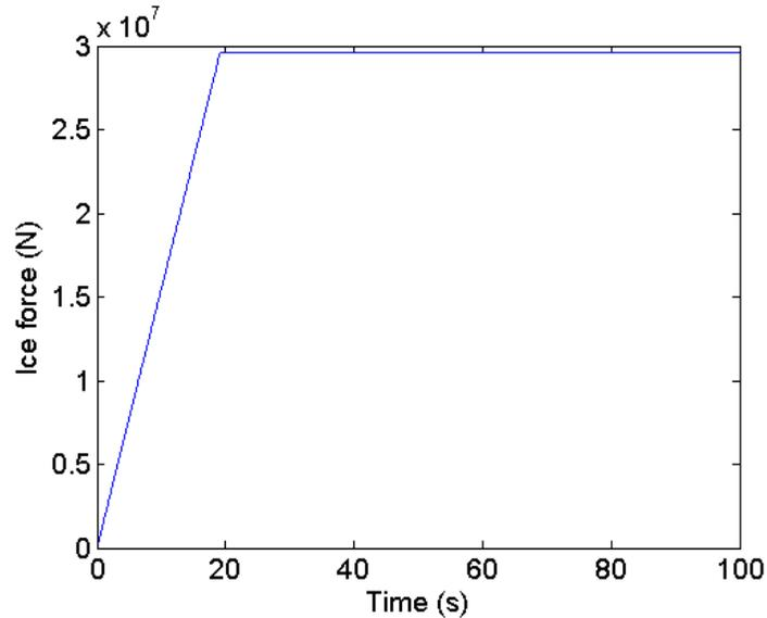
Figure 3 Ice load time history for ice model 1 sub-model 1
