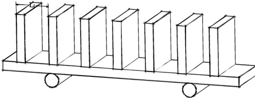
Figure 16 Ice teeth model of independent failure zones
