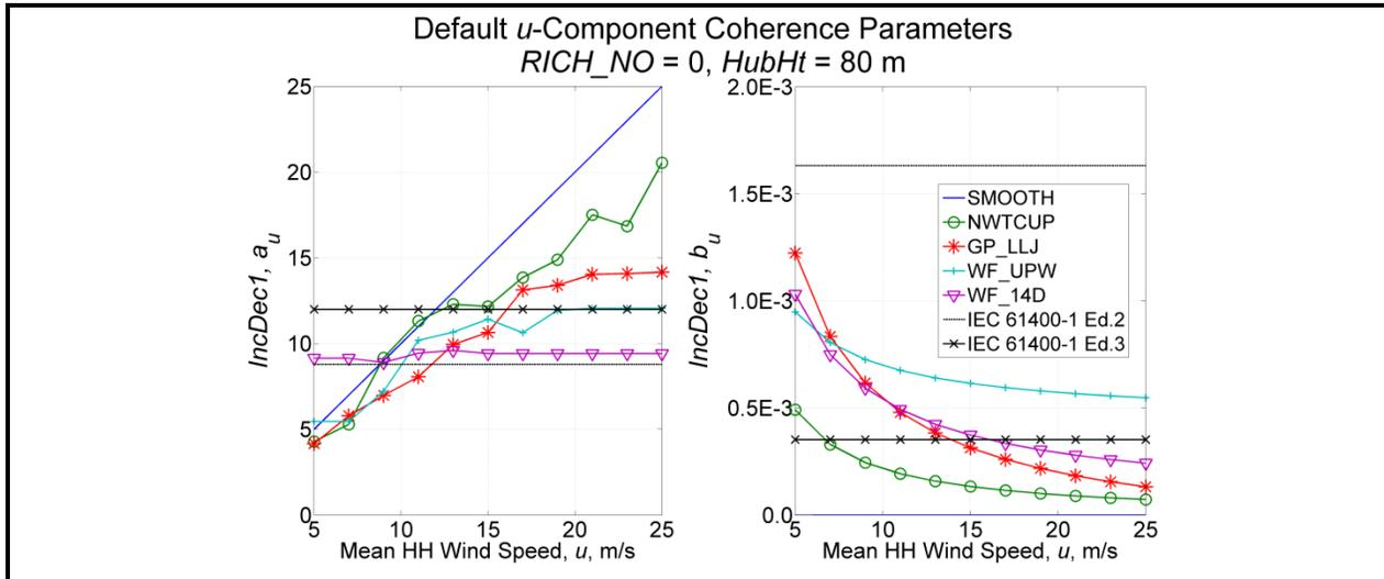
**Figure 13. Default  $u$ -component coherence parameters,  $IncDec1$ , ( $a_u$  left,  $b_u$  right) as a function of wind speed, using  $RICH\_NO = 0$  and  $HubHt = 80$  m (IEC values are plotted for comparison)**
