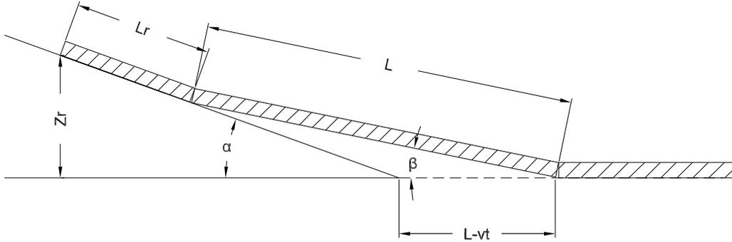
Figure 22 2D model of ice sheet riding up the cone
