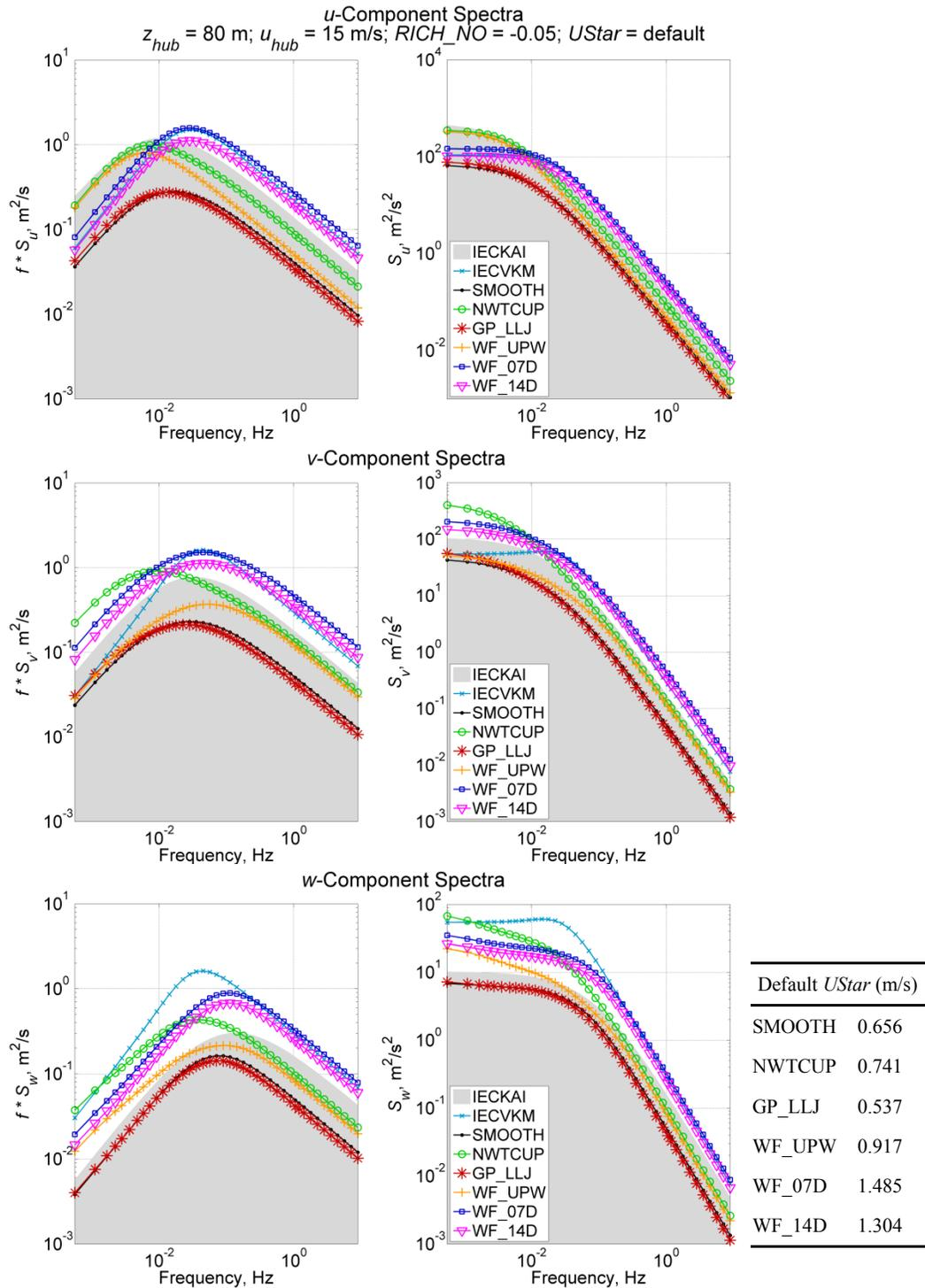
**Figure G-5. Unstable velocity spectra using a 15 m/s wind speed at 80 m; the non-IEC models use  $RICH\_NO = -0.05$  and  $UStar = \text{“default”}$ ; the IEC models, which are neutral ( $RICH\_NO = 0$ ), were added for reference; they use NTM category “B” and 61400-1 3<sup>rd</sup> ed. scaling**
