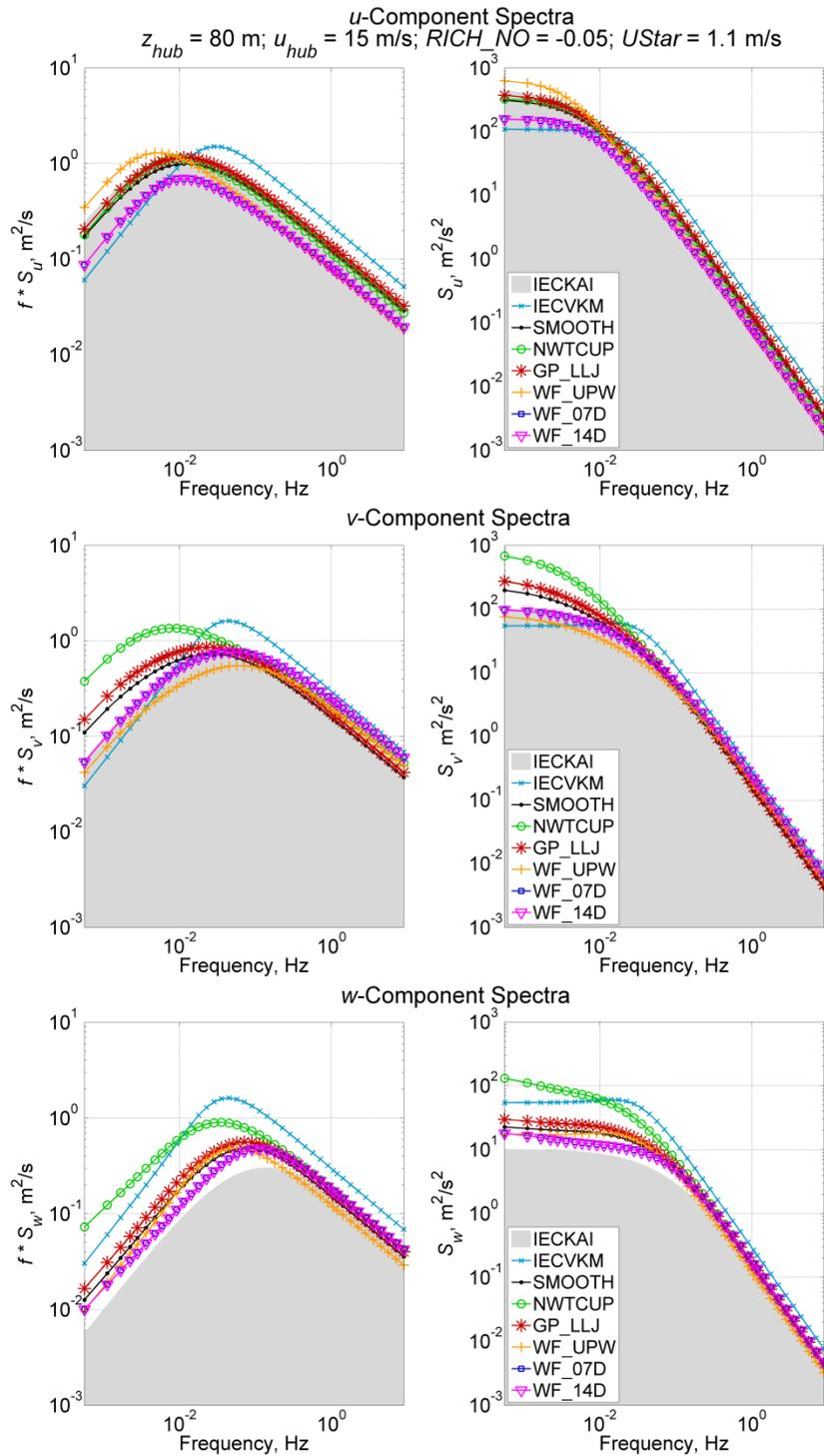
**Figure G-6. Unstable velocity spectra using a 15 m/s wind speed at 80 m; the non-IEC models use  $RICH\_NO = -0.05$  and  $UStar = 1.1 \text{ m/s}$ ; the IEC models, which are neutral ( $RICH\_NO = 0$ ), were added for reference; they use NTM category “B” and 61400-1 3<sup>rd</sup> ed. scaling**
