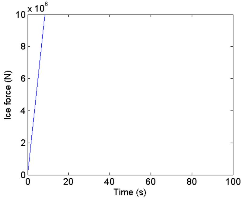
Figure 5 Ice load time history for ice model 1 sub-model 3
