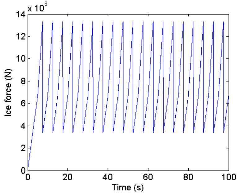
Figure 9 Ice load time history for ice model 2 sub-model 2
