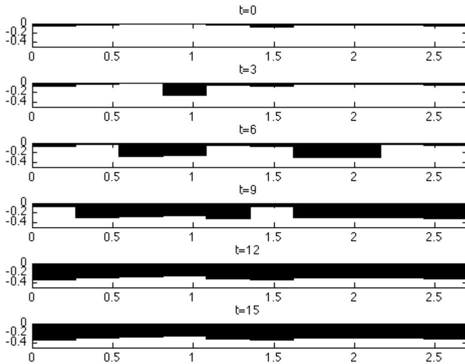
Figure 17 Ice-structure contact profile progressing over time
