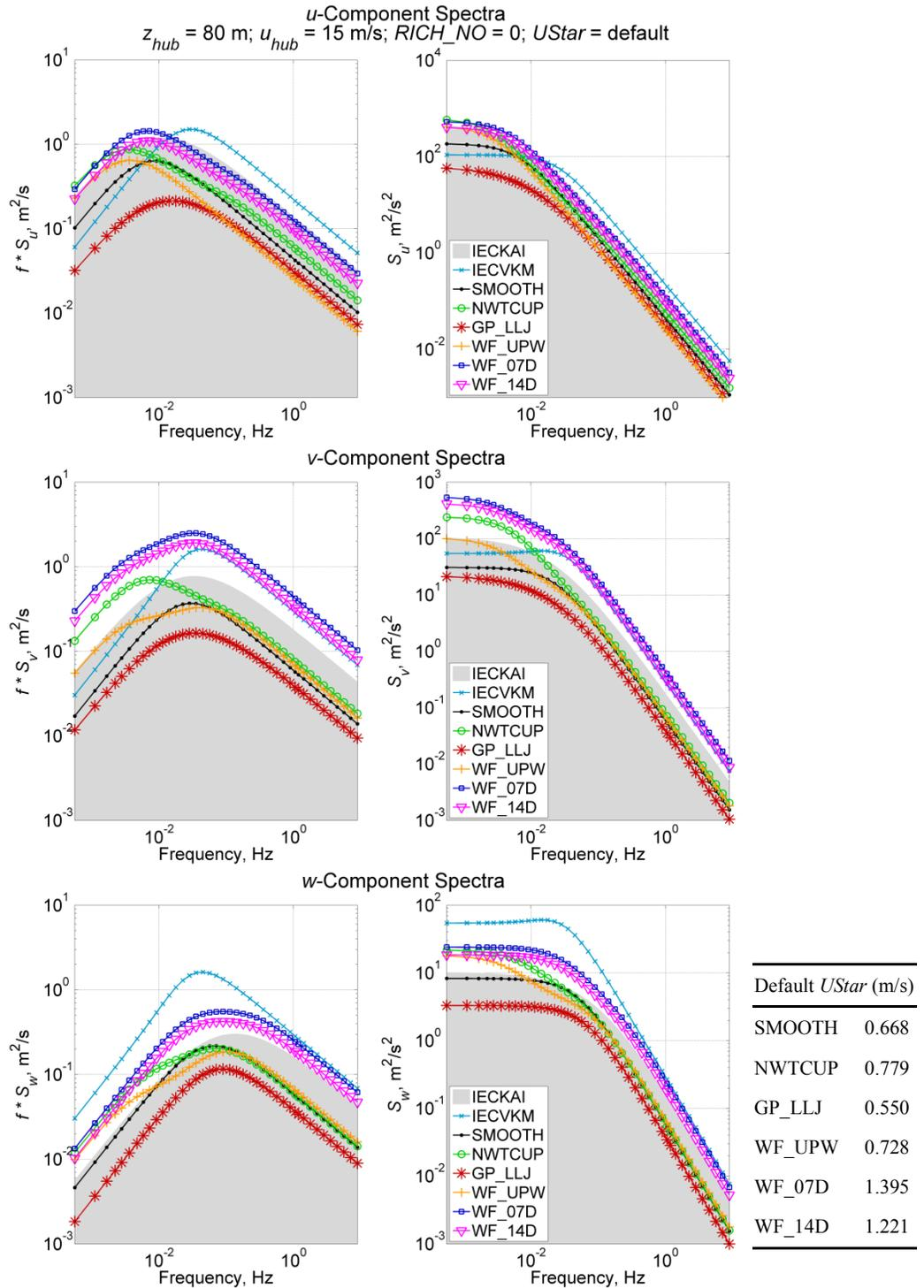
**Figure G-1. Neutral velocity spectra for the 8 spectral models available in TurbSim, using a 15 m/s wind speed at 80 m; IECKAI and IECVKM use NTM category “B” and 61400-1 3<sup>rd</sup> ed. scaling; the non-IEC models use  $RICH\_NO = 0$  and  $UStar = \text{“default”}$**
