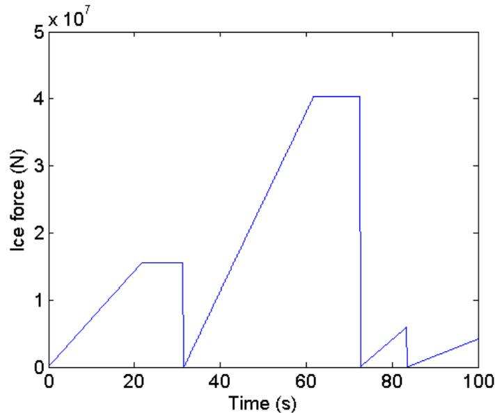
Figure 10 Ice load time history for ice model 3 sub-model 1
