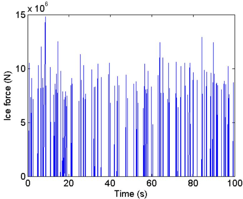
Figure 11 Ice load time history for ice model 3 sub-model 2
