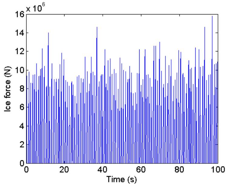
Figure 12 Ice load time history for ice model 3 sub-model 3
