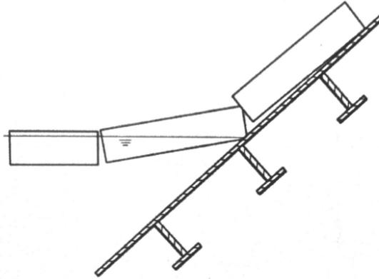
Figure 19 Ice bending on sloping structure (Sanderson 1988)
