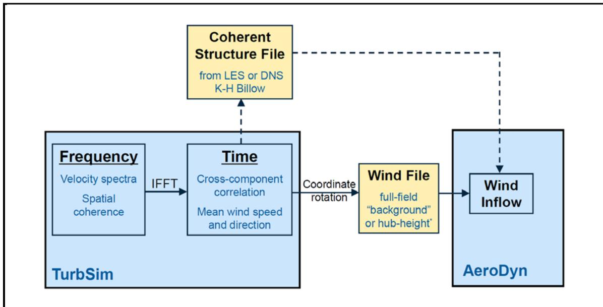
**Figure 1. TurbSim simulation method: a transformation from the frequency domain to time domain producing wind output compatible with InflowWind; optional coherent structures are written to a separate file and superimposed in AeroDyn v13 (they require a full-field background wind file)**
