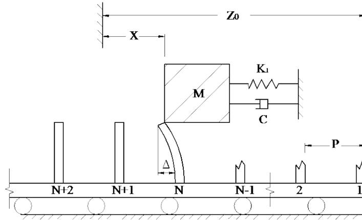
Figure 6 Ice-structure interaction model
