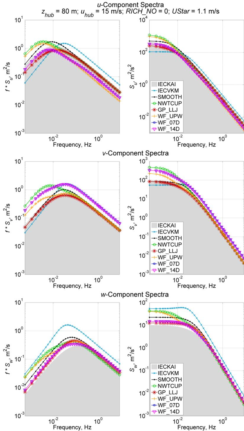
**Figure G-2. Neutral velocity spectra for the 8 spectral models available in TurbSim, using a 15 m/s wind speed at 80 m; IECKAI and IECVKM use NTM category “B” and 61400-1 3<sup>rd</sup> ed. scaling; the non-IEC models use  $RICH\_NO = 0$  and  $UStar = 1.1 \text{ m/s}$**
