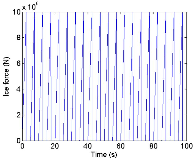
Figure 8 Ice load time history for ice model 2 sub-model 1
