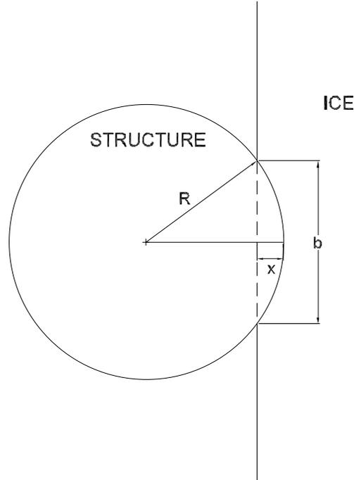
Figure 26 Ice structure interface
