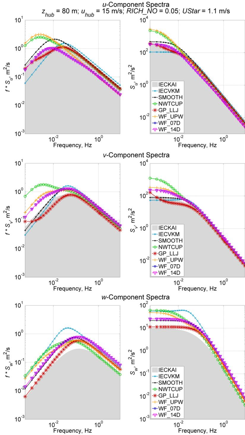
**Figure G-4. Stable velocity spectra using a 15 m/s wind speed at 80 m; the non-IEC models use RICH\_NO = 0.05 and UStar = 1.1 m/s; the IEC models, which are neutral (RICH\_NO = 0), were added for reference; they use NTM category “B” and 61400-1 3<sup>rd</sup> ed. scaling**
