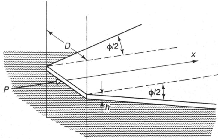
Figure 2 Wedge-shaped ice sheet floating on water (Sanderson 1988)
