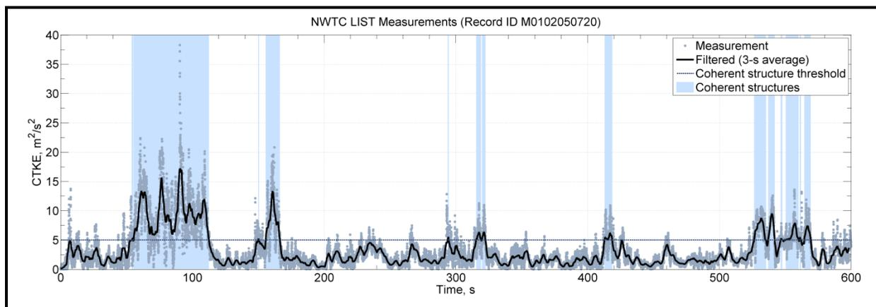
**Figure 25. Coherent structures in a 10-minute period from the NWTC LIST dataset: the time series shows the 3-s mean CTKE (solid black line) crossing the dashed threshold line, which indicates the location of the coherent structures (indicated in blue)**
