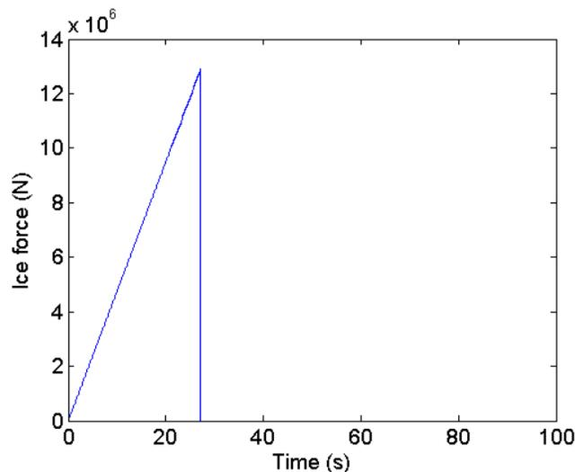
Figure 4 Ice load time history for ice model 1 sub-model 2
