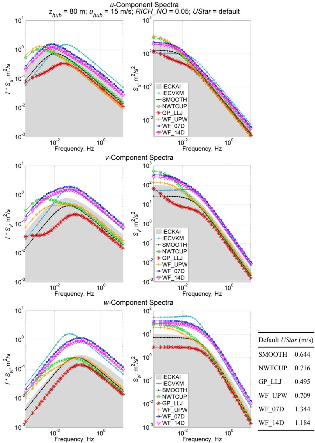
**Figure G-3. Stable velocity spectra using a 15 m/s wind speed at 80 m; the non-IEC models use  $RICH\_NO = 0.05$  and  $UStar = \text{“default”}$ ; The IEC models, which are neutral ( $RICH\_NO = 0$ ), were added for reference; they use NTM category “B” and 61400-1 3<sup>rd</sup> ed. scaling**
