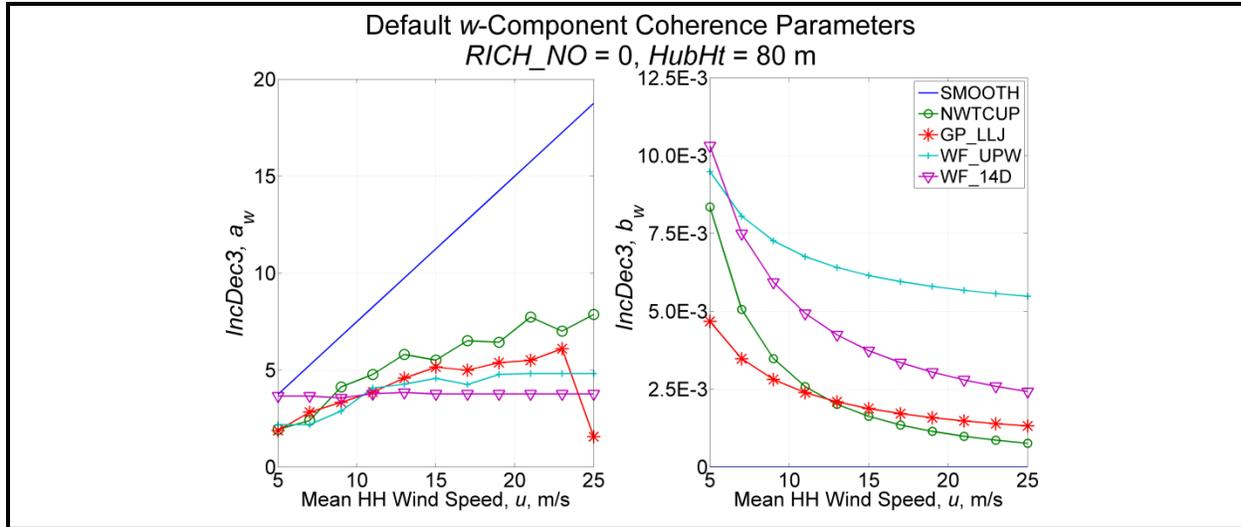
**Figure 15. Default  $w$ -component coherence parameters,  $IncDec3$ , ( $a_w$  left,  $b_w$  right) as a function of wind speed, using  $RICH\_NO = 0$  and  $HubHt = 80$  m (IEC does not define  $w$ -component coherence parameters)**
