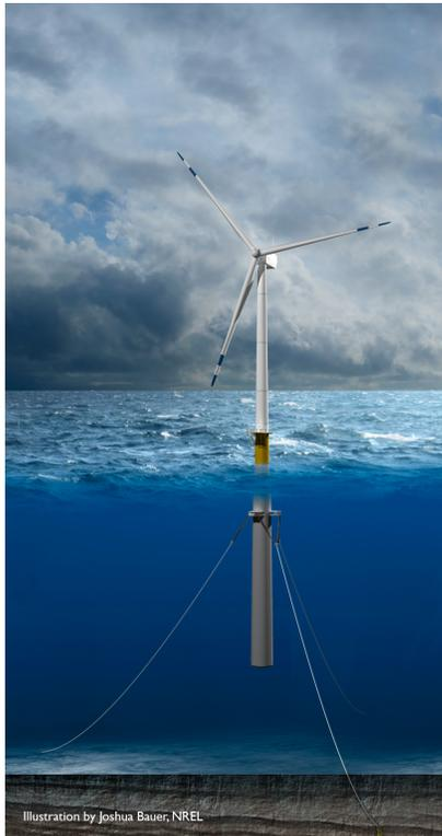
FIG. 1. *The spar platform pictured illustrates a practical use for a multisegmented line in floating offshore wind turbines. The bridle joint provides additional yaw stiffness, an essential component for dynamic stability.*
