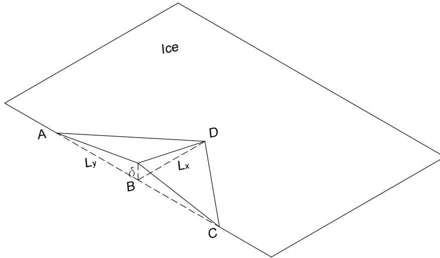
Fig 21. Geometry of the approximate ice displacement field
