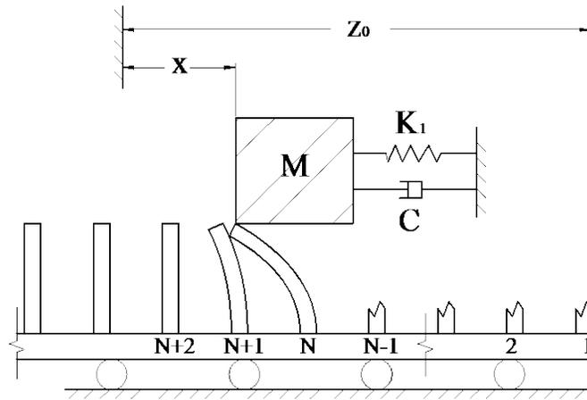
Figure 7 Ice-structure interaction with two ice teeth bending
