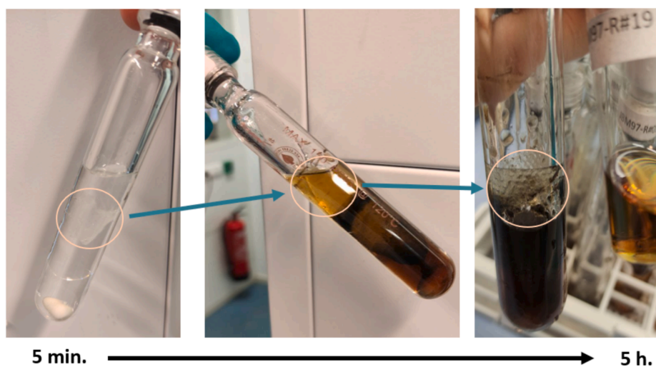
Fig. 6. Visual inspection of the reactor during the conversion of cellulose-containing wipes to CMF. The reactor contained Montvale wipes in 1 mL of 42 wt% HCl and 3 mL of chlorobenzene. The mixture was first stirred at room temperature for 16 h (middle picture) and then for 5 h at 80 °C, replacing the organic phase every hour during heating. The transparent polypropylene residue is visible after collecting the organic phase (right picture, in circle).
