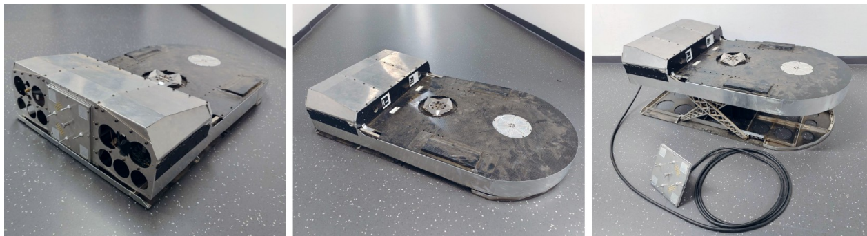
Fig. 3. TMDS rear (left) and front view (centre) folded as well as in extended state (right) with partially uncoiled tether.
