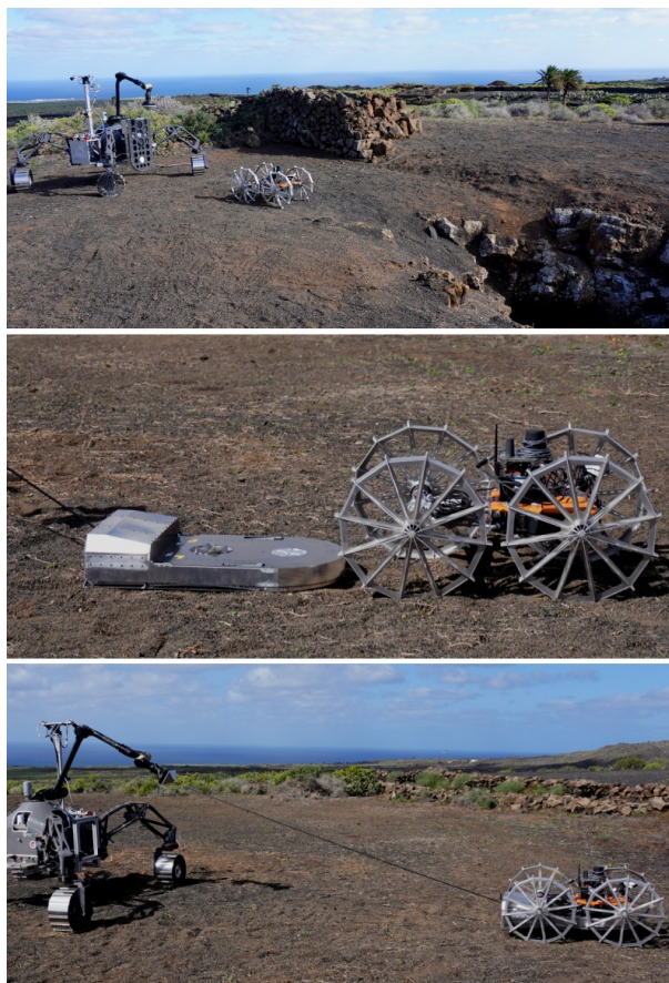
Fig. 9. The two rovers, Coyote3 and SherpaTT, with the TMDS during TMDS Deployment (top), Docking Behavior (centre) and start of Rappelling Rover Guidance (bottom).
