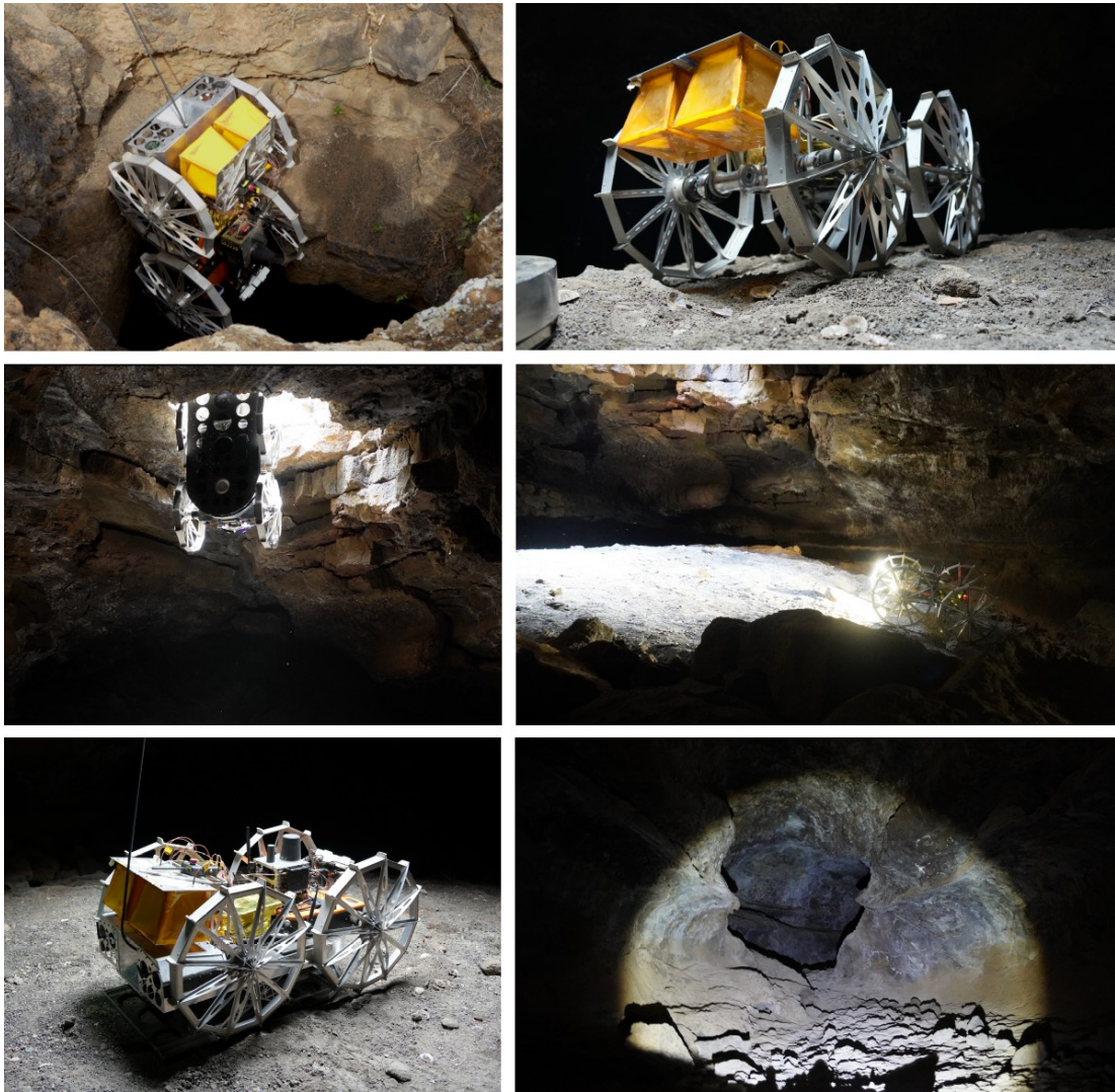
Fig. 10. Coyote3 starts the descent through the skylight (1), rappels down the vertical walls (2), reaches the bottom of the lava tube (3), undocks from the TMDS (4) and begins the subsurface lava tube exploration (5-6).
