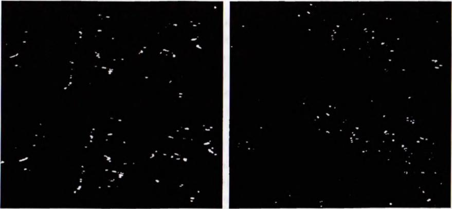
Fig. 2. Examples of HSCI images; the image sector is  $27 \times 36 \text{ cm}^2$ ; wind speeds: left: 2.4 m/s; right: 6.4 m/s. The top half of each image represents the first field, the bottom half the second field (time difference: 17ms).
