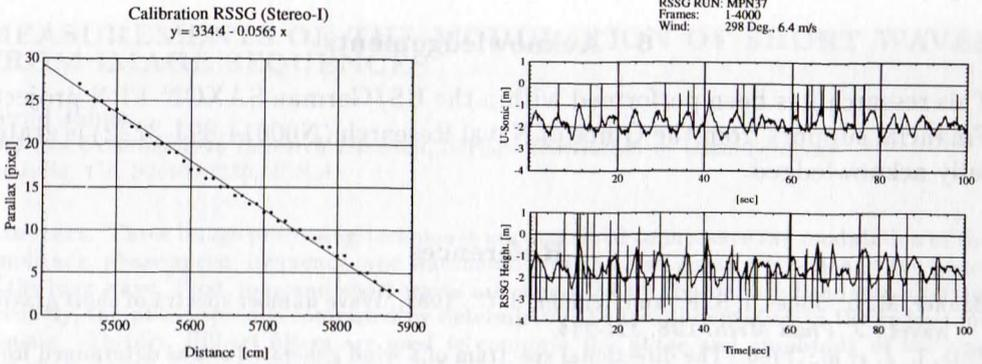
Fig. 3. Left: Calibration with an artificial target. Right: Comparison of the stereo data with an ultrasonic distance sensor. Some drop-outs in the height measurements occur when zero or only very few reflections are contained in the image.
