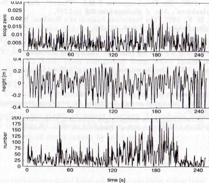
Fig. 4. Top: Probability for slope of zero measured as part of the surface area covered by the reflections. Middle: Time series of the wave height averaged over the image sector of  $40 \times 30 \text{ cm}^2$ . Two frames have been taken per s; the wind speed was 2.5 m/s. Bottom: Time series of the number of reflections in the stereo images.
