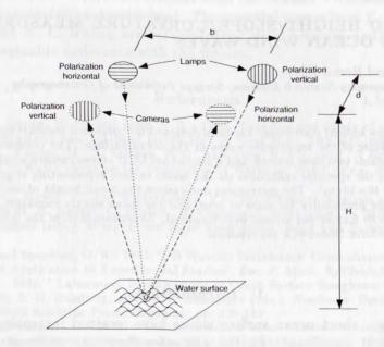
Fig. 1. Illustration of the principle of the height/slope/curvature instrument (HSCI).
