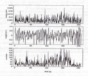
Fig. 4. Top: Probability for slope of zero measured as part of the surface area covered by the reflections. Middle: Time series of the wave height averaged over the image sector of  $40 \times 30 \,\mathrm{cm}^2$ . Two frames have been taken per s; the wind speed was  $2.5 \,\mathrm{m/s}$ . Bottom: Time series of the number of reflections in the stereo images.
