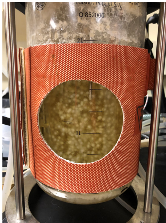
Fig. 4. G. tsugae fermented in a bioreactor after 7 days of fermentation.
