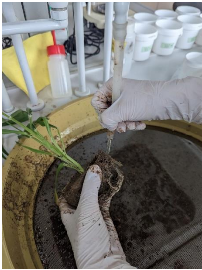
2 Bulk soil removal by gentle rinsing
