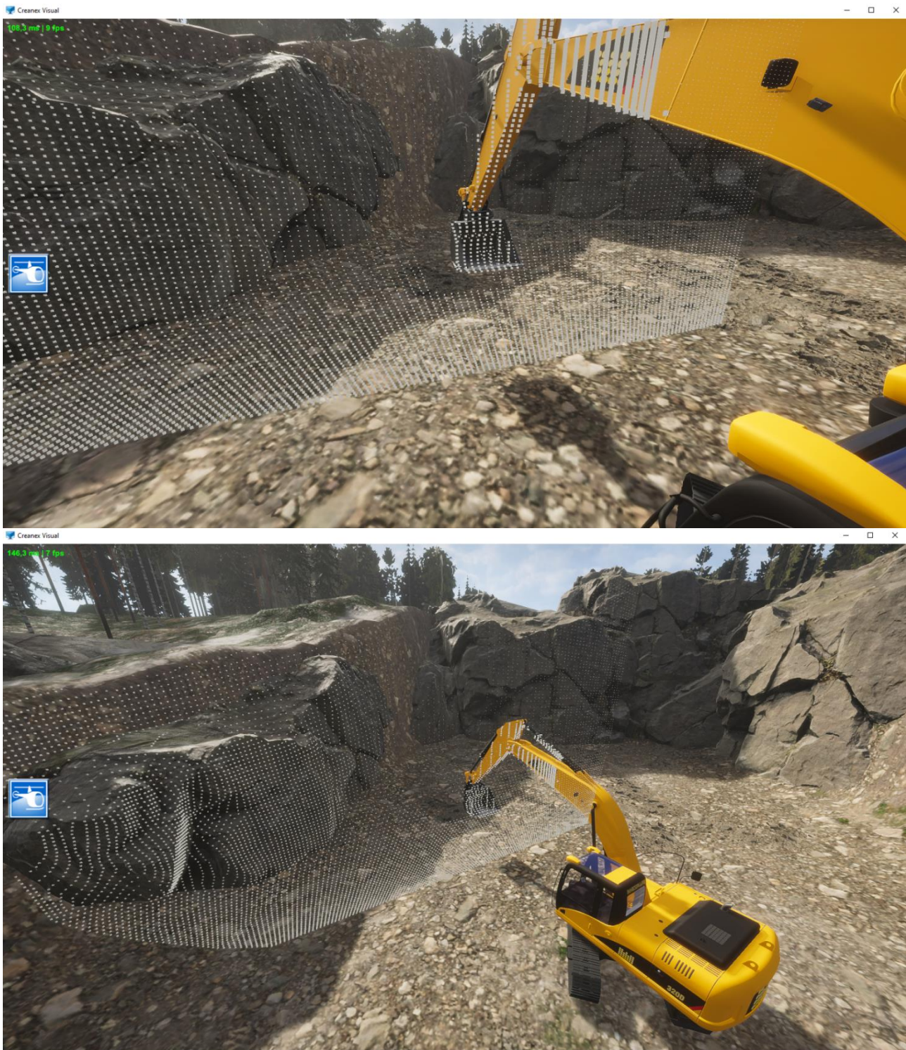
Figure 35: LIDAR data visualized on top of standard visual view. Distance data from Unity depth buffer.
