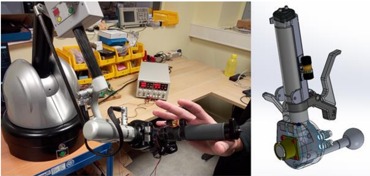
Figure 5: Prototype of Virtuose TREH handle with vibrotactor attached.
