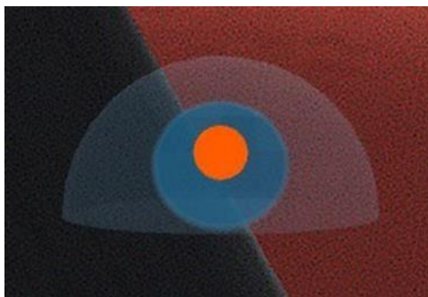
Figure 19: Screenshot of the hand tracking feedback feature. The sphere is currently orange because no hands are being tracked.
