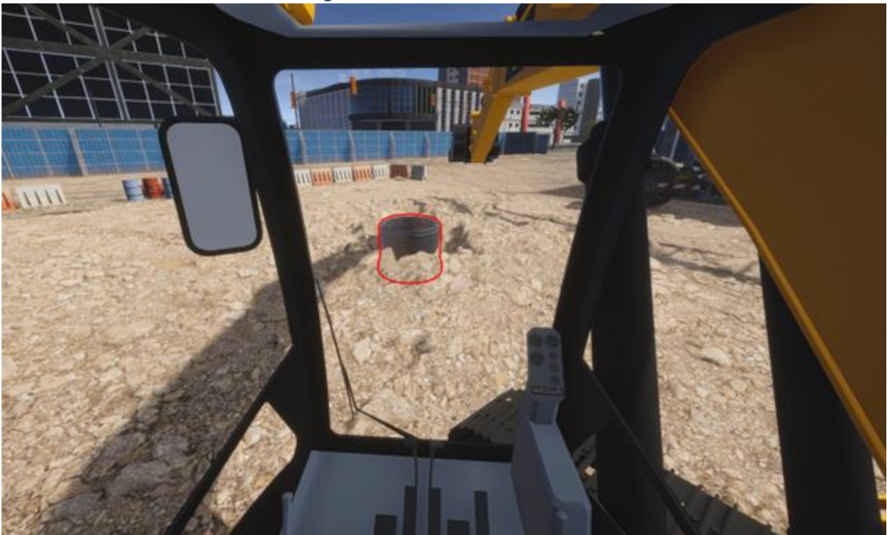
Figure 33: Underground obstacle highlighted in excavation area.
