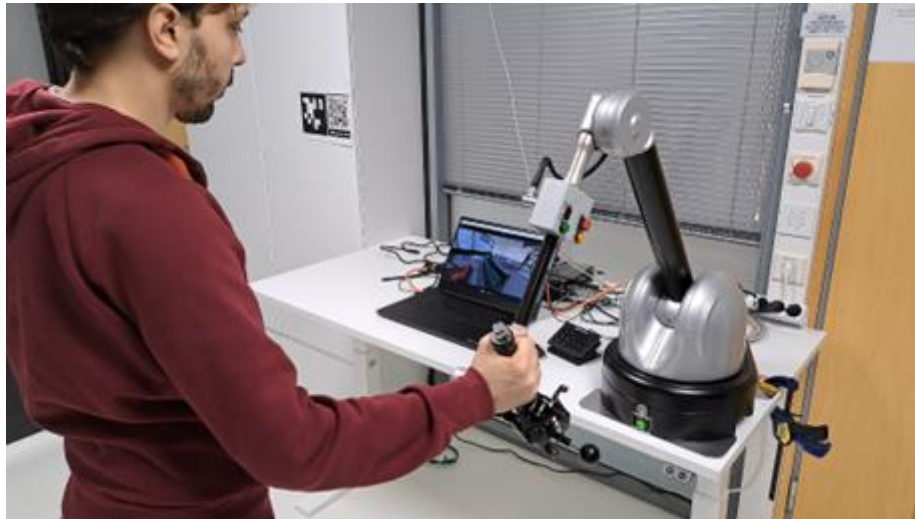
Figure 16: Integrating a Virtuose6D haptic interface with the UC2 simulator
