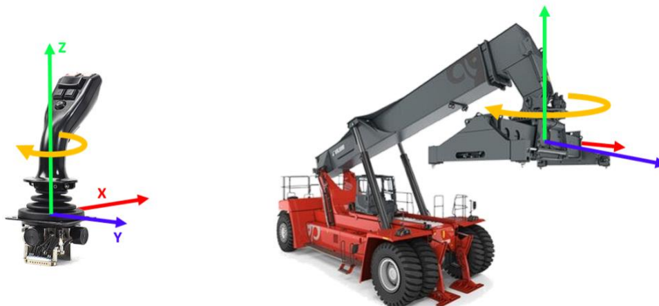
Figure 23: Concept for direct position control of the spreader with a 4DoF joystick
