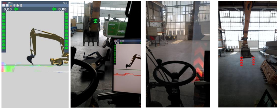
Figure 39: Different modalities to visualize the correct digging depth (3D-model, LED-matrix display, HUD, augmented video-stream)
