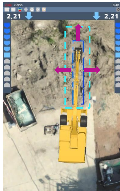
Figure 35 Visualization of the trench model (blue outline), projected on the terrain model
