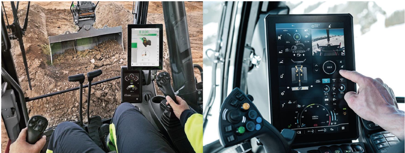
Figure 2: Examples for off-highway vehicle cabin screens (left: excavator; right: snow groomer)
