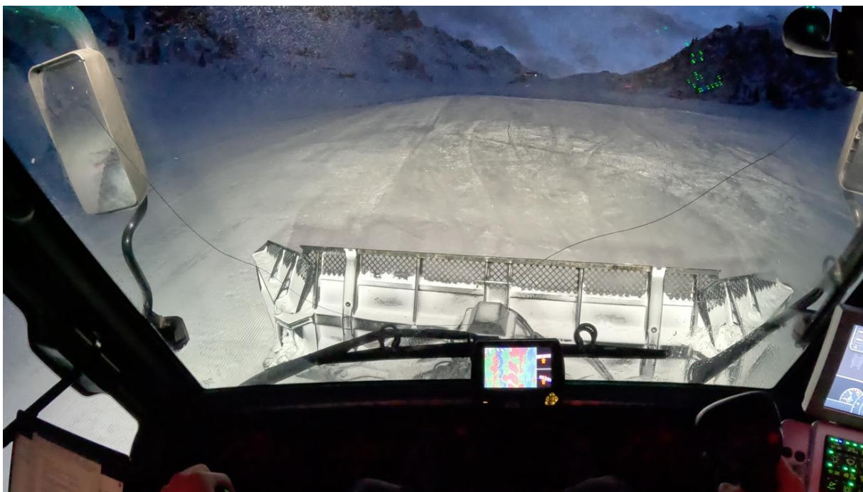
Figure 3: Snow-groomer cabin view. Snow depth measurement system screen in the bottom middle.
