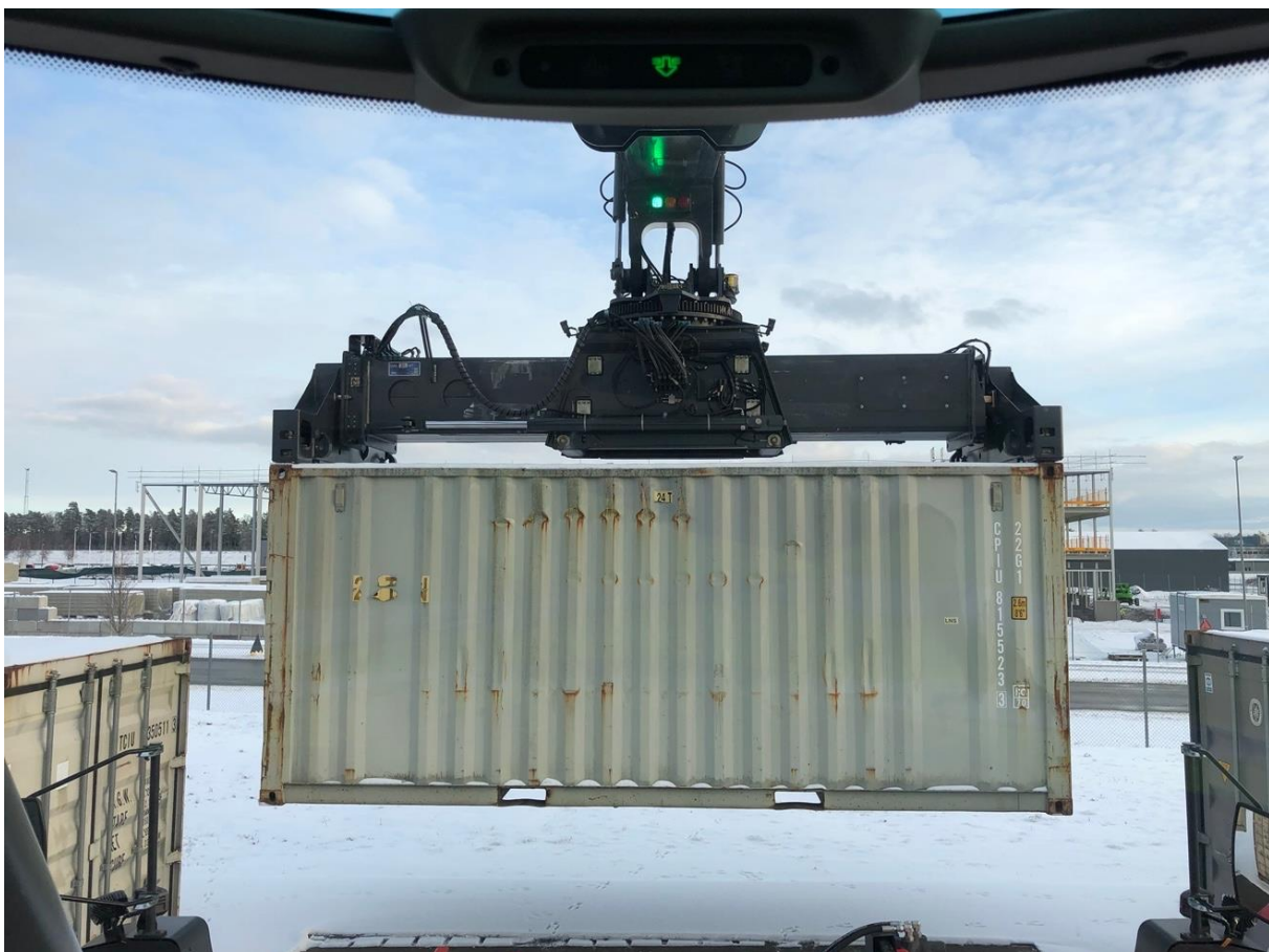
Figure 10: Reachstacker cabin view, spreader visible in the center. Green lights indicate locked twist locks.
