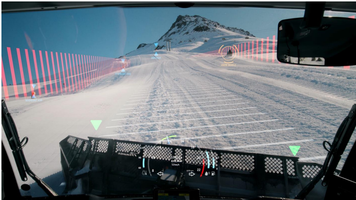
Figure 7 Potential scenario of a snowgroomer operator view using XR-technology ©PRINOTH
