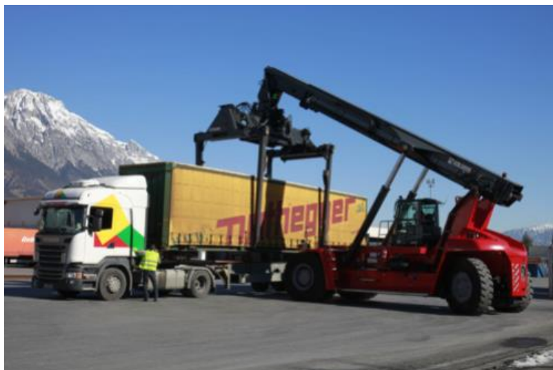
Figure 18: Reachstacker picking container from the trailer ©KALMAR
