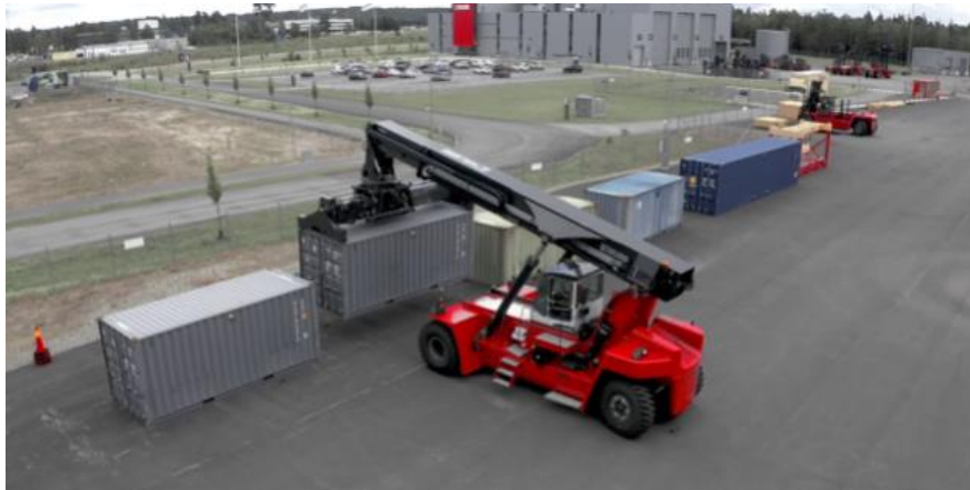
Figure 17: Reachstacker placing container to the ground ©KALMAR
