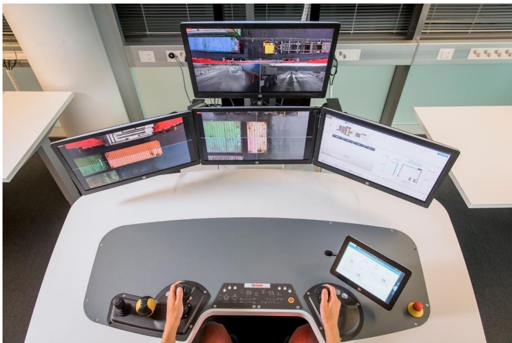
Figure 12: Kalmar Remote Control Desk ©KALMAR
