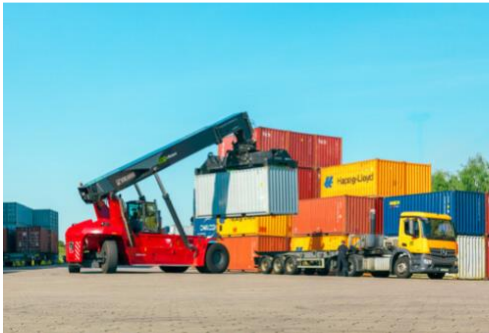
Figure 19: Reachstacker placing container to the trailer ©KALMAR
