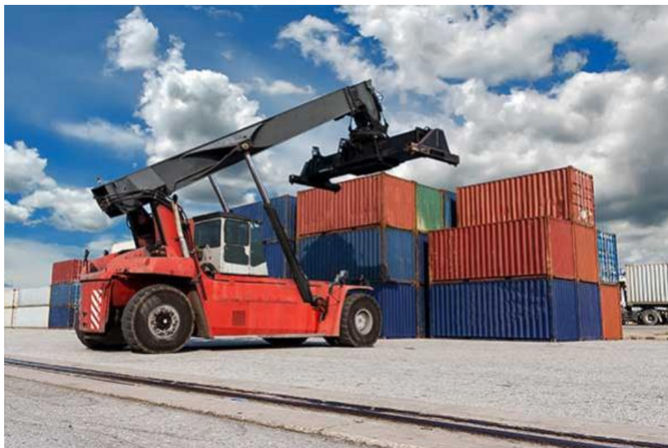
Figure 13: Reachstacker picking container from stack ©KALMAR
