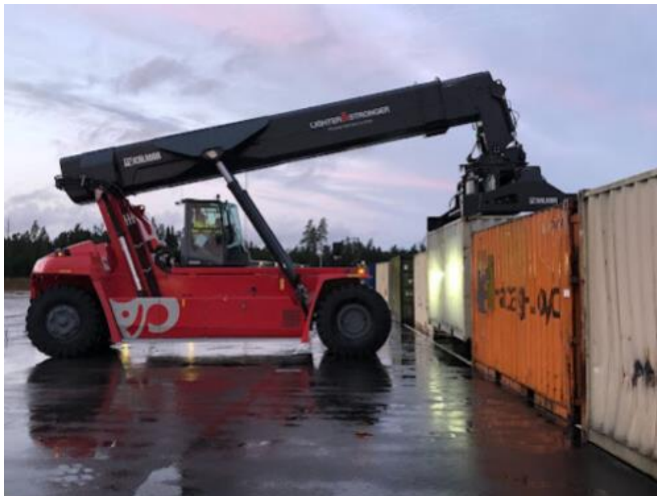
Figure 16: Reachstacker picking container from the ground. ©KALMAR
