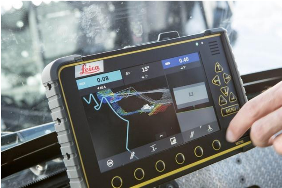
Figure 4 Snowgroomer interface touch screen for snow measurement ©PRINOTH
