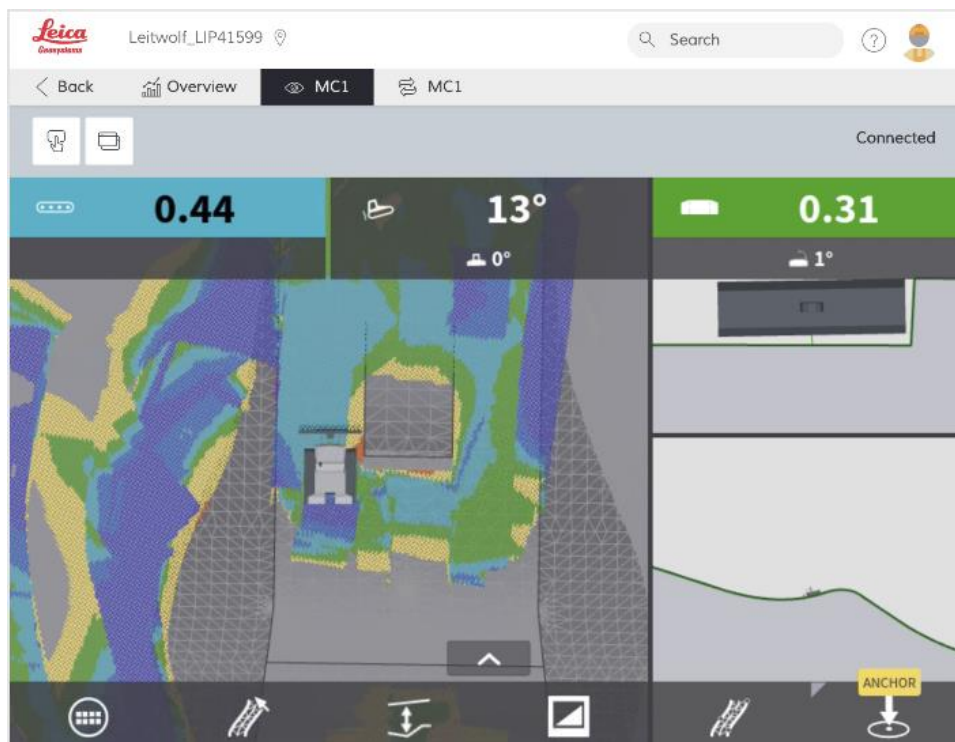
Figure 6 Touch screen showing top, side and blade view ©PRINOTH
