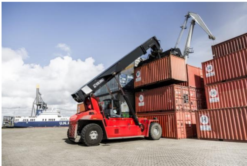
Figure 15: Reachstacker placing container to the stack ©KALMAR
