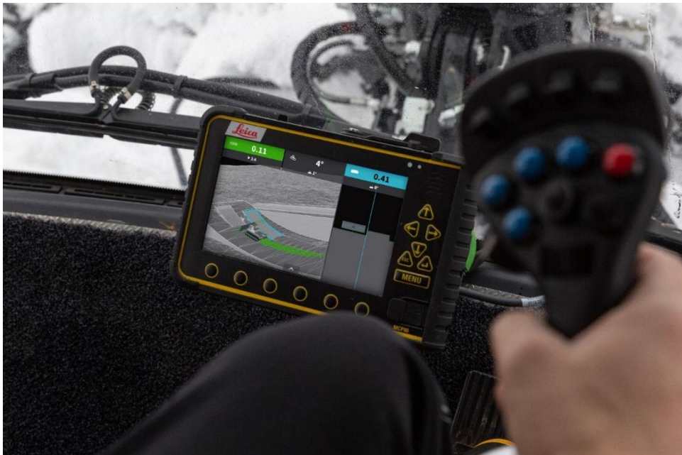
Figure 5 Touch screen showing a 3D park model target surface ©PRINOTH
